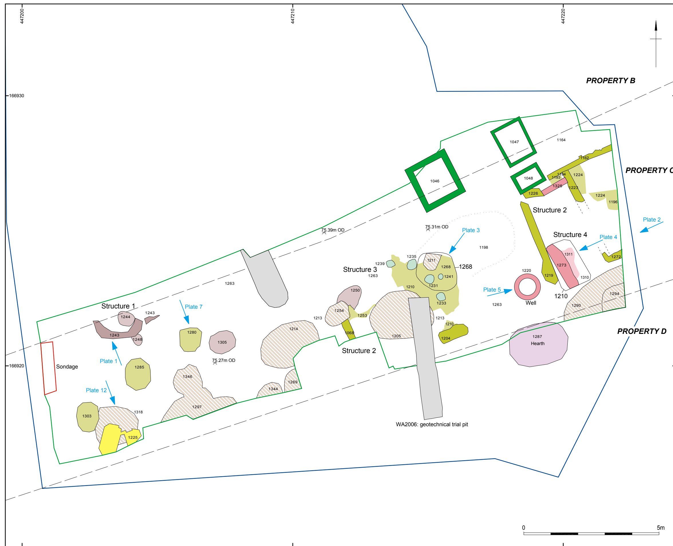
Plan of Stage 2 (deeper excavation area) showing main structural elements
