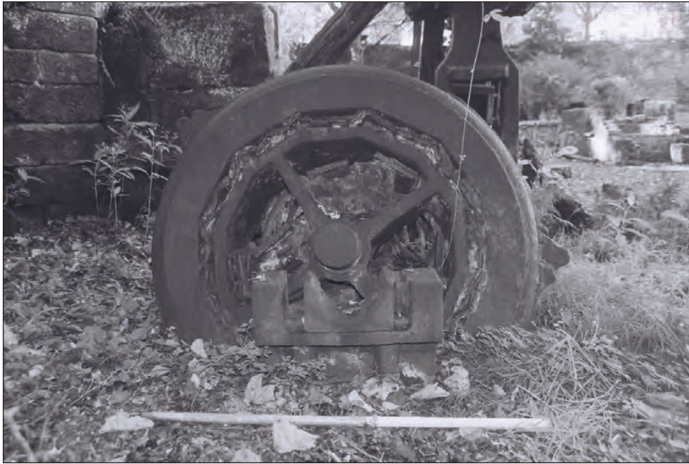
Plate 67: Detail of the cam wheel at the west end of the east helve hammer, south end of the central phase 1 former forge building (Film 9.26)
