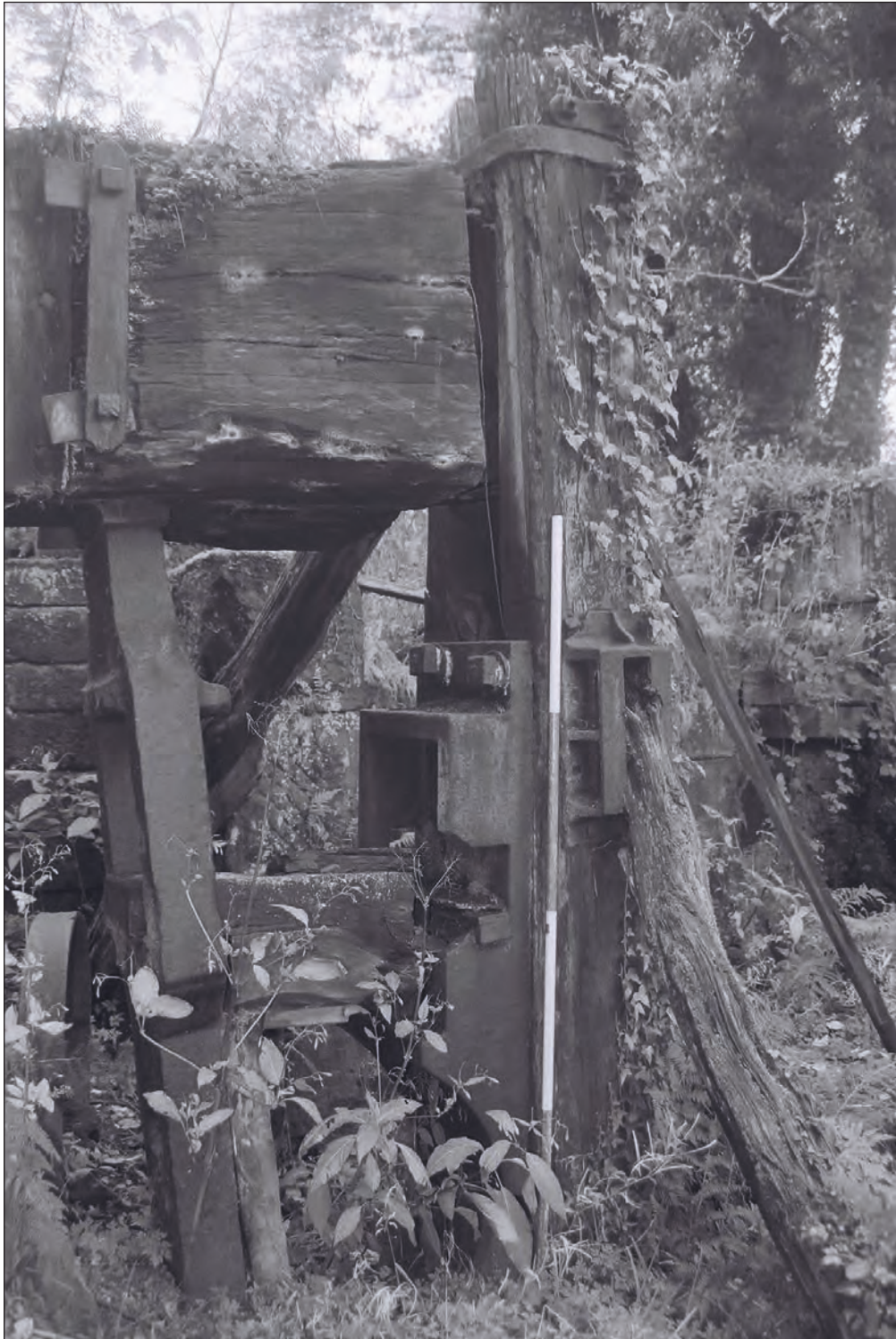
Plate 64: Detail of the west end of the east helve hammer, south end of the central phase 1 former forge building (Film 9.3)
