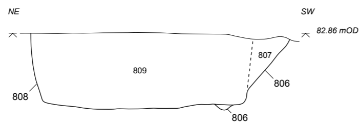
South-east facing section of pit 808 and ditch 806
