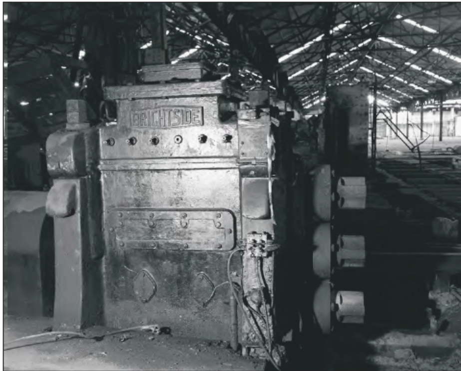
Plate 51: Detail of the 'Brightside' branded gear box from the 18" Rolling Mill. (film 23.02)
