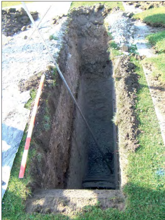
Plate 19: Tidworth: Test pit 1568 from the east, showing made-ground over original ground surface
