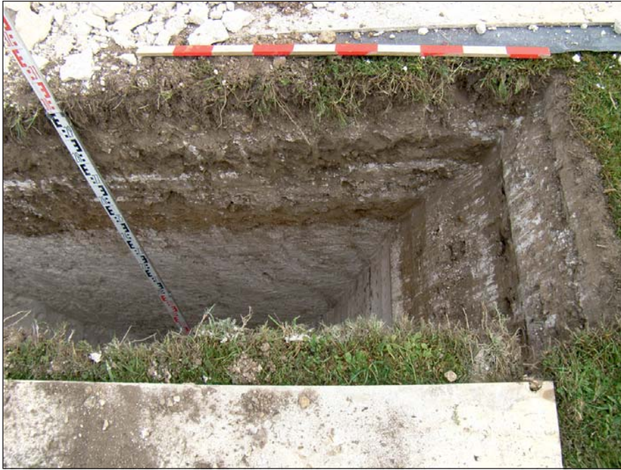
Plate 18: Tidworth: Test pit 1539 from the south, showing series of made-ground deposits
