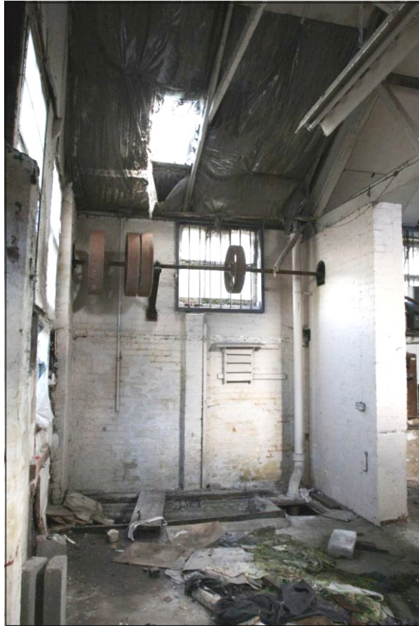
Plate 11: Building 3 north-west corner of the interior with laundry drive shaft and wheels still in-situ
