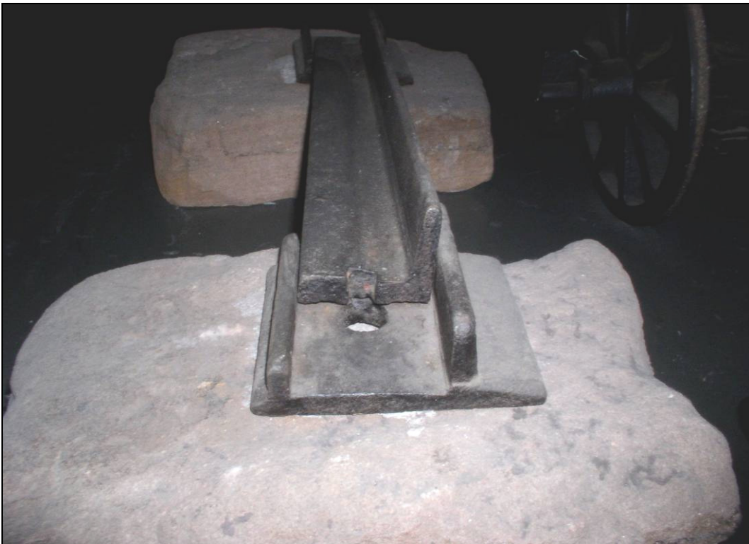
Plate 29 – Example of tramway sleeper pad and rail fixtures (photograph from ARCUS archive, original source unknown)
