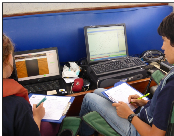
Plate 13: Data acquisition – sidescan sonar (left) and navigation (right)
