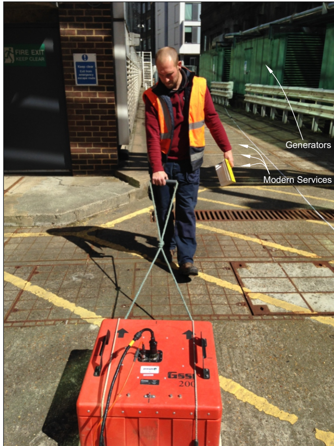
Plate 1: Modern Services in the eastern part of the survey area leading from the generators to the building
