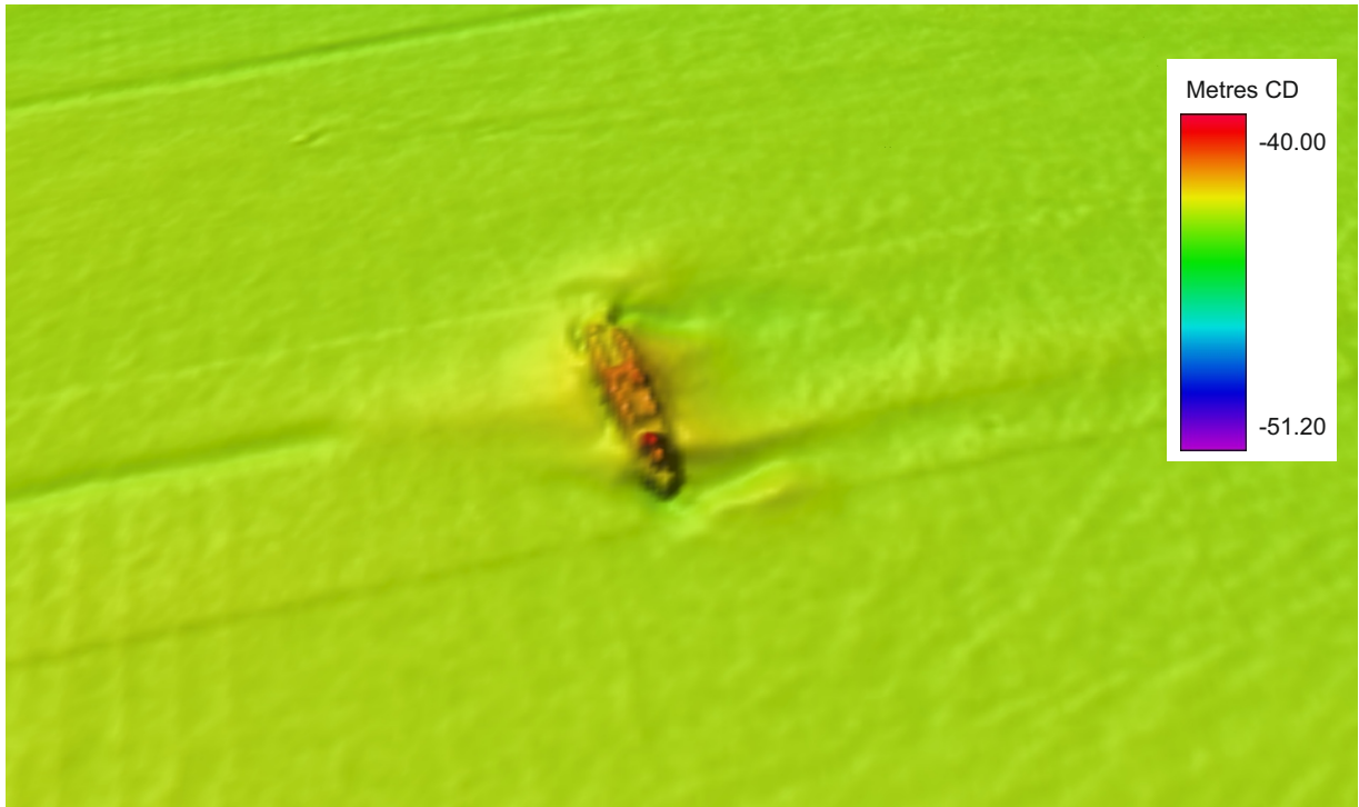
Multibeam echosounder image of wreck 7004 (x1 vertical exaggeration), facing north
