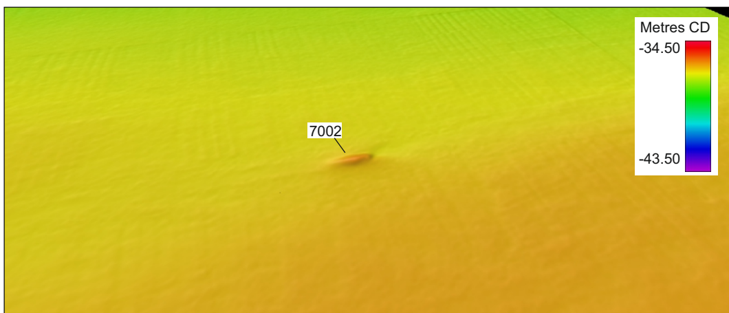
Multibeam echosounder image of mound 7002 (x1 vertical exaggeration), facing north
