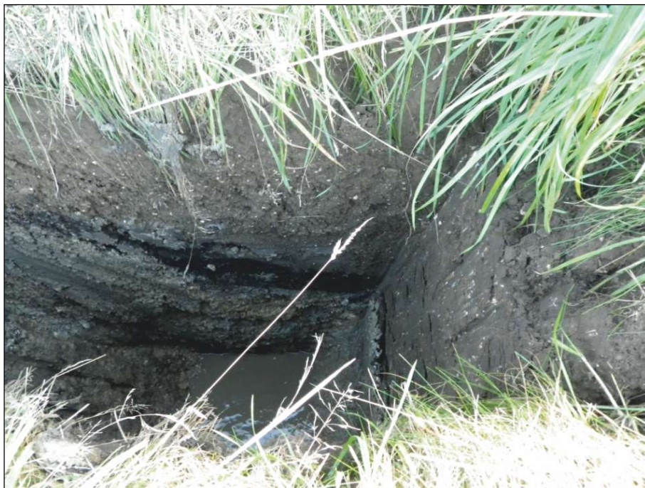
Plate 4: Test pit TP12 showing a black peat deposit (1204) located above the natural chalky gravel
