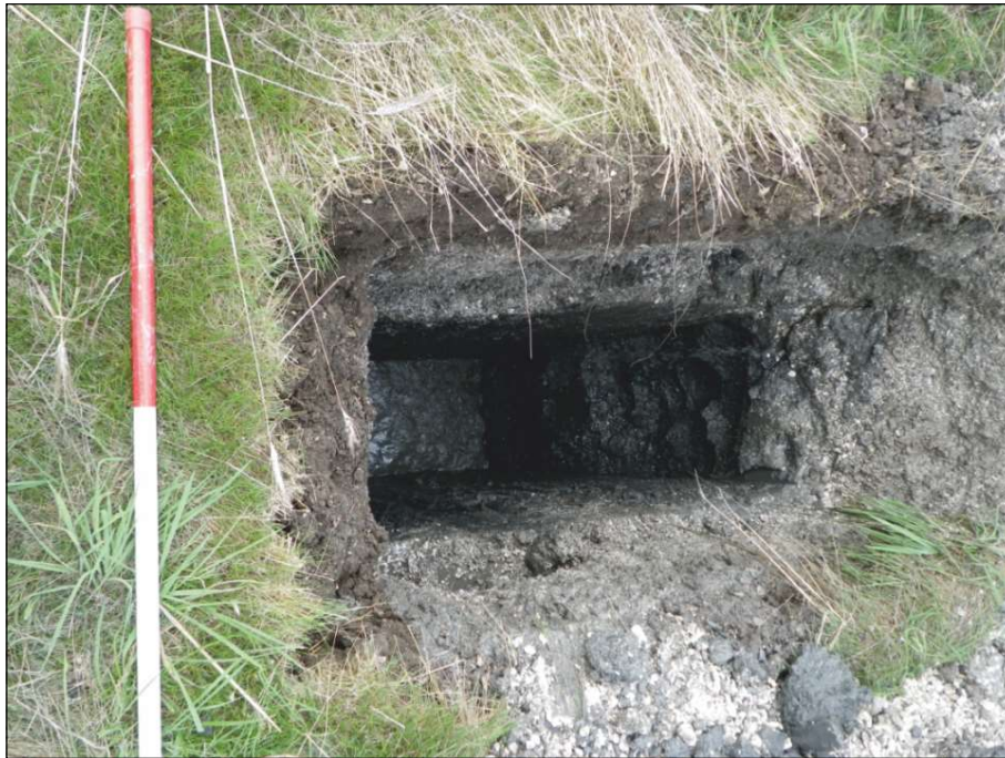
Plate 3: Test pit TP07 showing the natural chalky gravel and the decayed mudstone below
