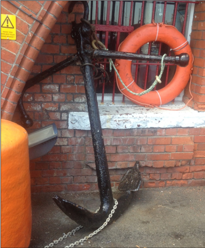
Plate 2: MAG_6854 Iron anchor Admiralty Pattern type
