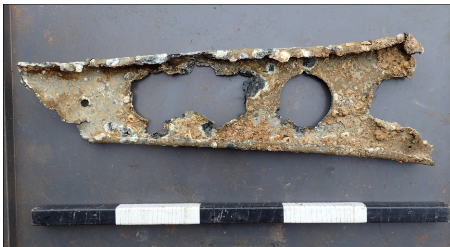
Plate 6: MAG_4959 Rib from either the rudder, elevator, aileron, or tailplane of a multi-engine aircraft
