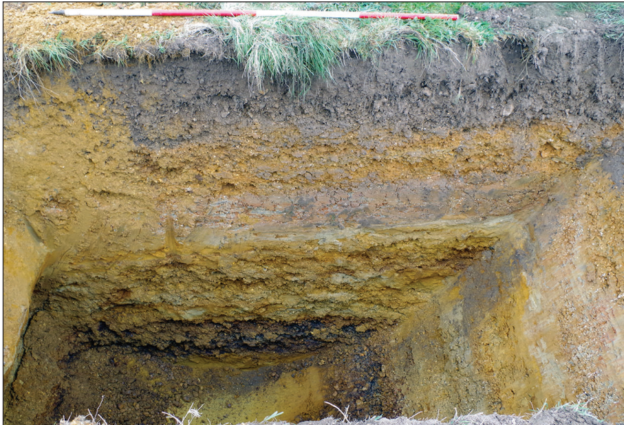
Plate 2 : TP 32 north-north-east facing section illustrating Selsey Sand Formation overlain by Phase I: river terrace and Phase II: 'Head brickearth' deposits
