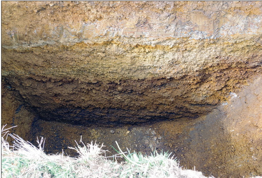
Plate 4: TP 33 detail of lower part of north-east facing section illustrating Phase I: river terrace deposits, overlain by Phase II: 'Head brickearth' deposits.
