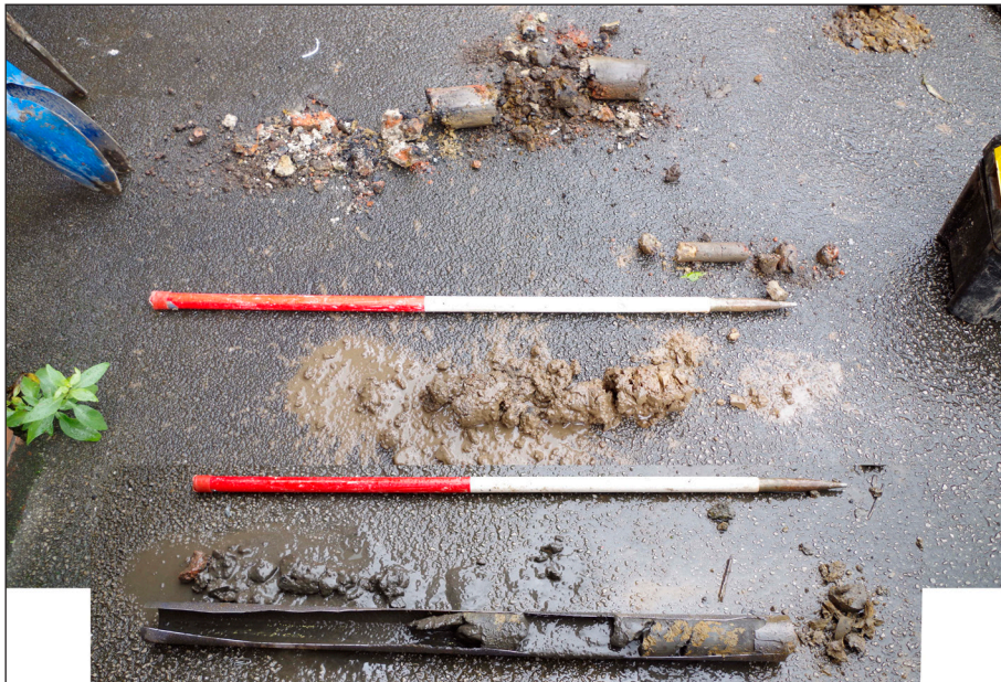
Plate 20: BH 11, drilling core, depth 1.2–2.0 m, 2.0–3.0 m, 3.0–4.0 m (from the top)
