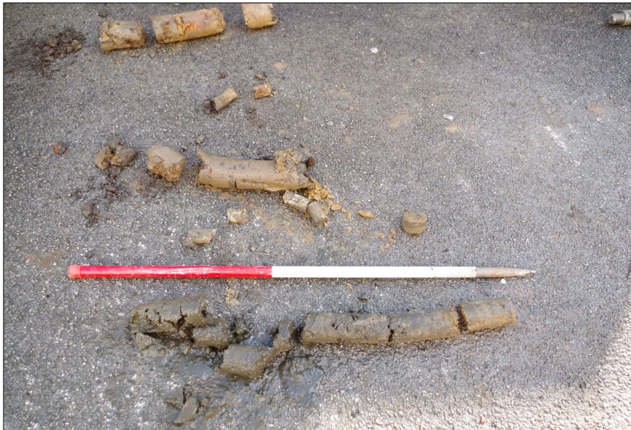
Plate 22: BH 12, drilling core, depth 1.2–2.0 m, 2.0–3.0 m, 3.0–4.0 m (from the top)
