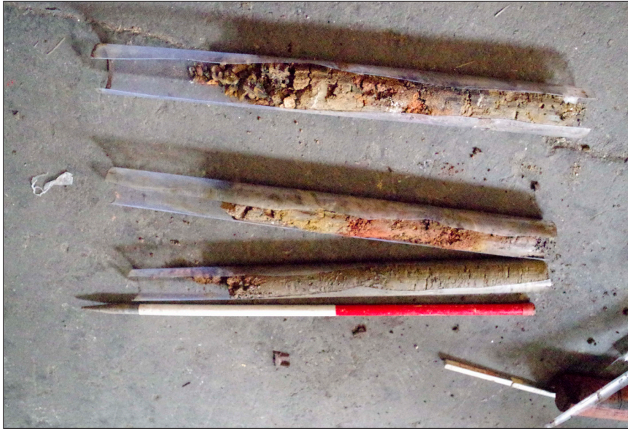
Plate 17: BH 9, drilling core, depth 1.2–2.0 m, 2.0–3.0m, 3.0–4.0 m (from the top)
