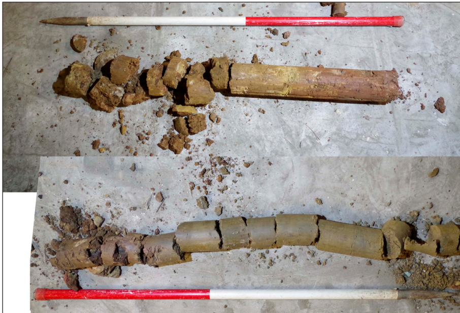
Plate 6: BH 3, drilling core, depth 1.2–2.0 m, 2.0–3.0 m (from the top)
