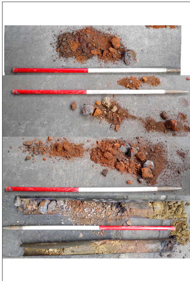
Plate 14: BH 7, drilling core, depth 1.2–2.0 m, 2.0–3.0 m, 3.0–4.0 m, 4.0–5.0 m, 5.0–6.0 m (from the top)
