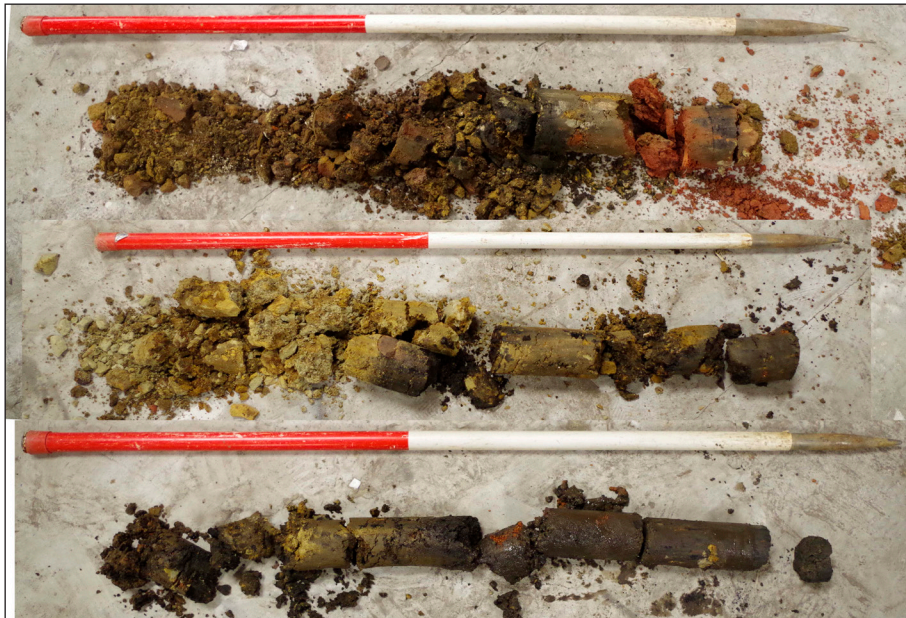
Plate 2: BH 1, drilling core, depth 1.2–2.0 m, 2.0–3.0 m, 3.0–4.0 m (from the top)
