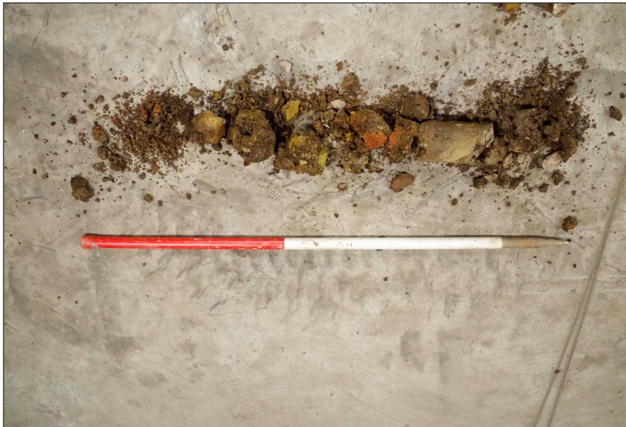
Plate 4: BH 2, drilling core, depth 1.2–2.0 m
