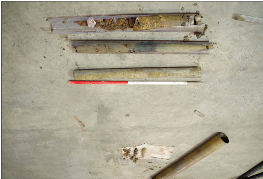
Plate 26: BH 15, drilling core, depth 1.2–2.0 m, 2.0–3.0 m, 3.0–4.0 m (from the top)
