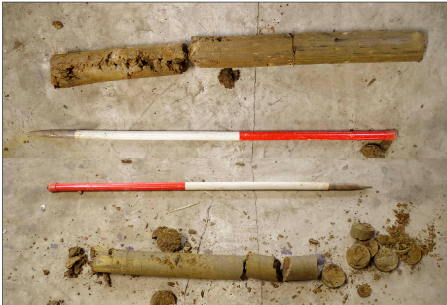
Plate 8: BH 4, drilling core, depth 1.2–2.0 m, 2.0–3.0 m
