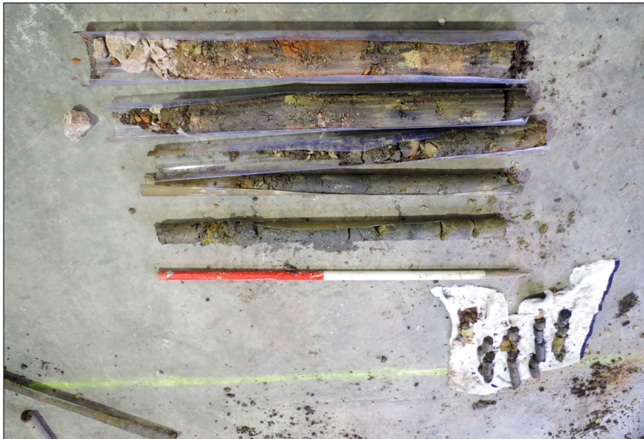
Plate 10: BH 5, drilling core, depth 1.2–2.0 m, 2.0–3.0 m, 3.0–4.0 m, 4.0–5.0 m, 5.0–6.0 m (from top to bottom)
