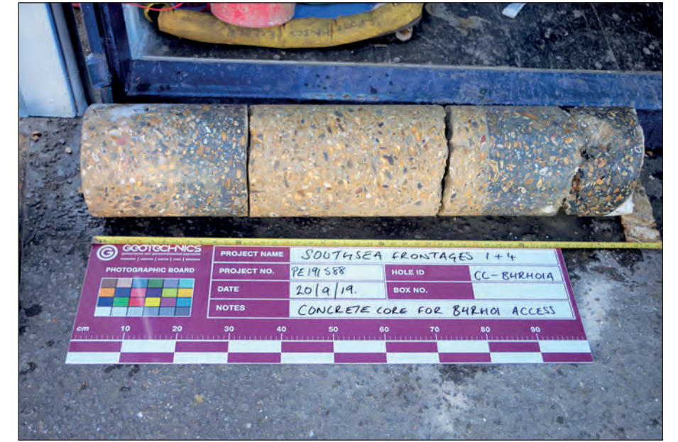
Plate 3: Concrete core from Trench 2
