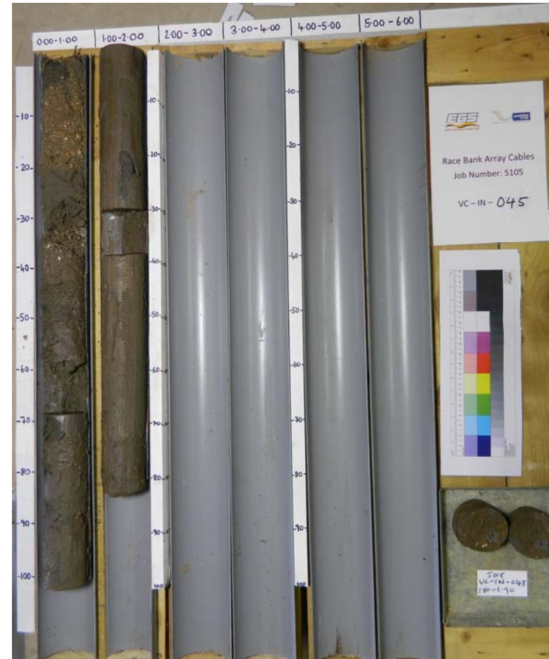
VC-IN-45. Seabed deposits over Glacial till with area of rooting at top of till.
