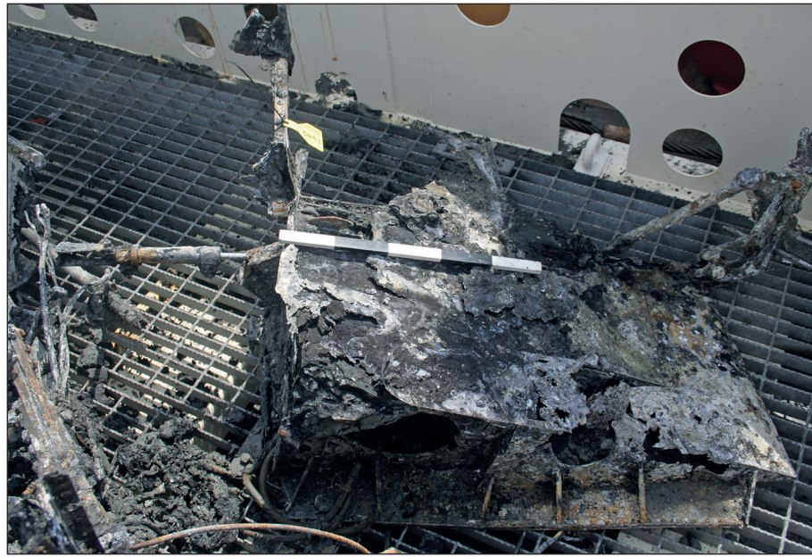
Plate 36: Inboard section of trailing edge of port wing with hydraulic ram
