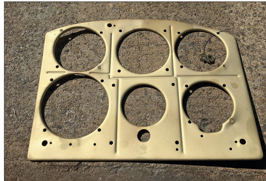
Plate 85: Cleaned blind flying panel © Tony Jupp
