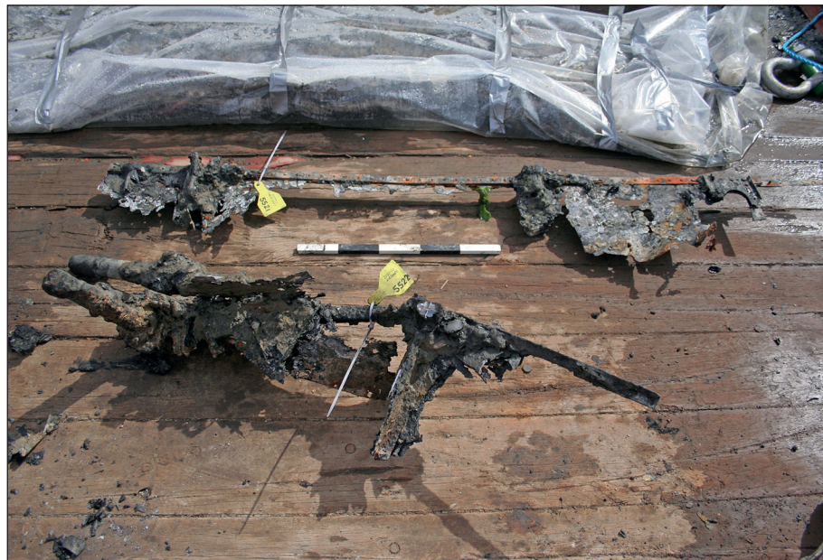
Plate 4: Starboard wing fragment- remains of front spar (5521) and support tubing at the inboard end of the wing (5522)
