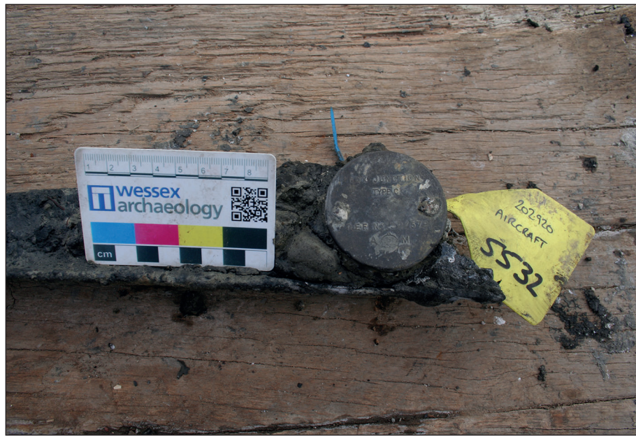
Plate 11: Air Ministry standard Bakelite electrical fitting
