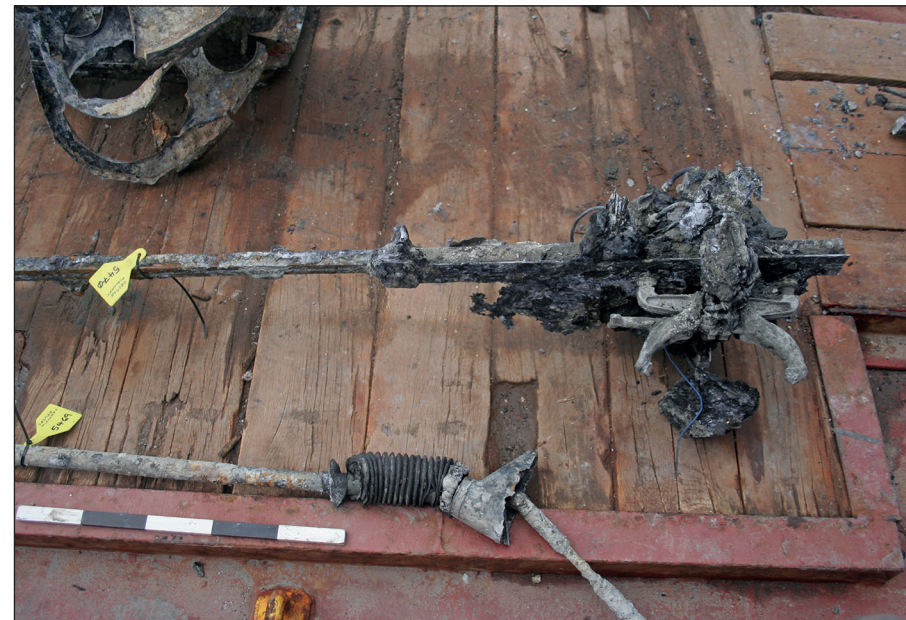
Plate 40: Bomb clutch on front spar of port wing
