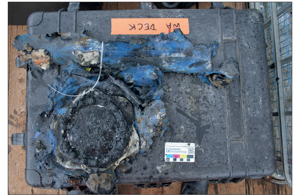
Plate 13: Starboard inboard tank fabric and inlet valve
