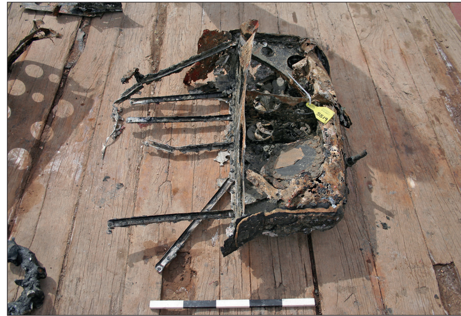
Plate 2: Starboard wing fragment- inboard fuel tank
