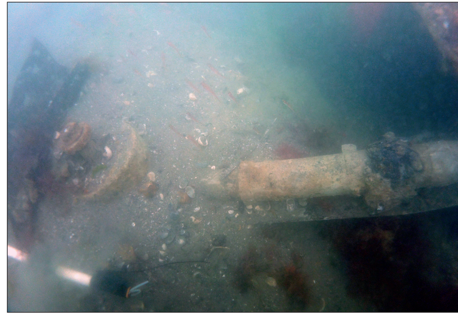
Plate 32: Starboard landing gear in half raised position on seabed
