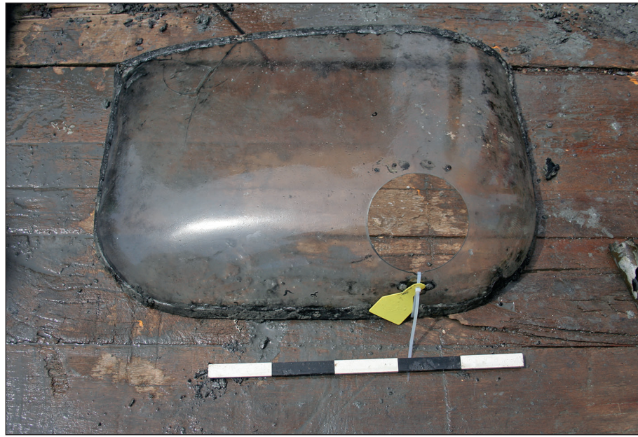
Plate 71: Starboard observers domed side window
