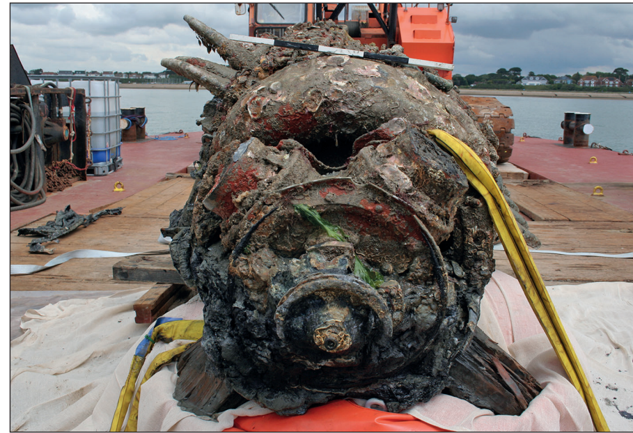
Plate 17: Rolls Royce Merlin 32 engine- front view showing 4 bladed propeller hub without spinner
