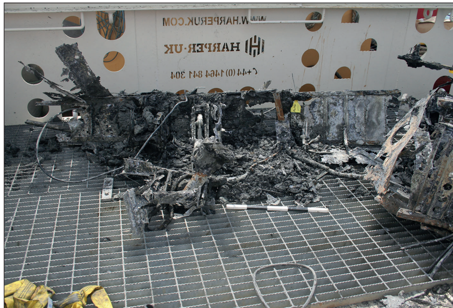
Plate 39: Section of port wing rear spar with internal fittings and ram for Youngman Flap
