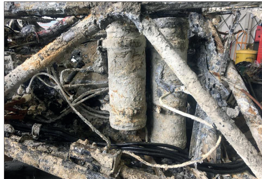
Plate 30: Hydraulic accumulators in the port wing stub © Tony Jupp
