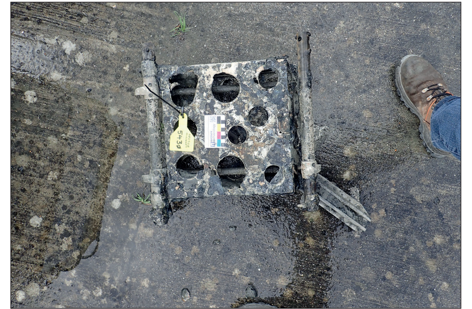
Plate 83: Base of pilot's seat with earlier variant mounting
