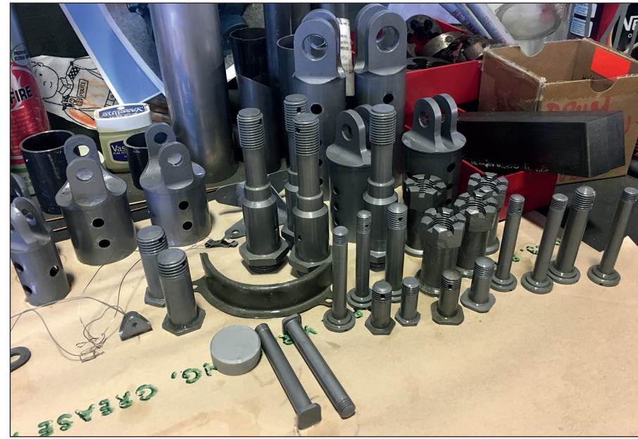
Plate 92: Cleaned and conserved tube fittings from Pilot's cockpit © Tony Jupp
