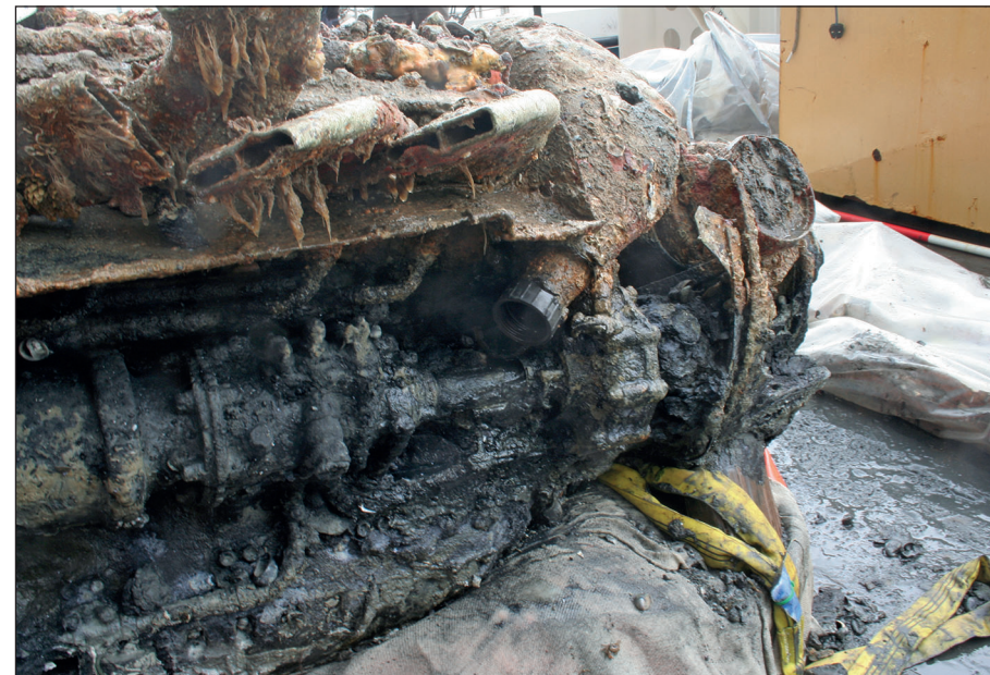
Plate 20: Starboard side of engine showing high degree of preservation
