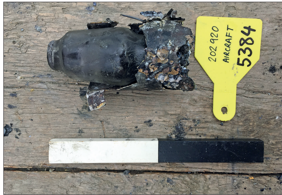
Plate 57: Glass radio valve
