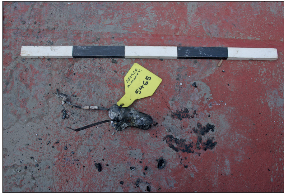
Plate 61: Cell lamp with cable label
