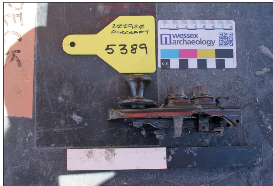
Plate 59: Morse key from TAG cockpit
