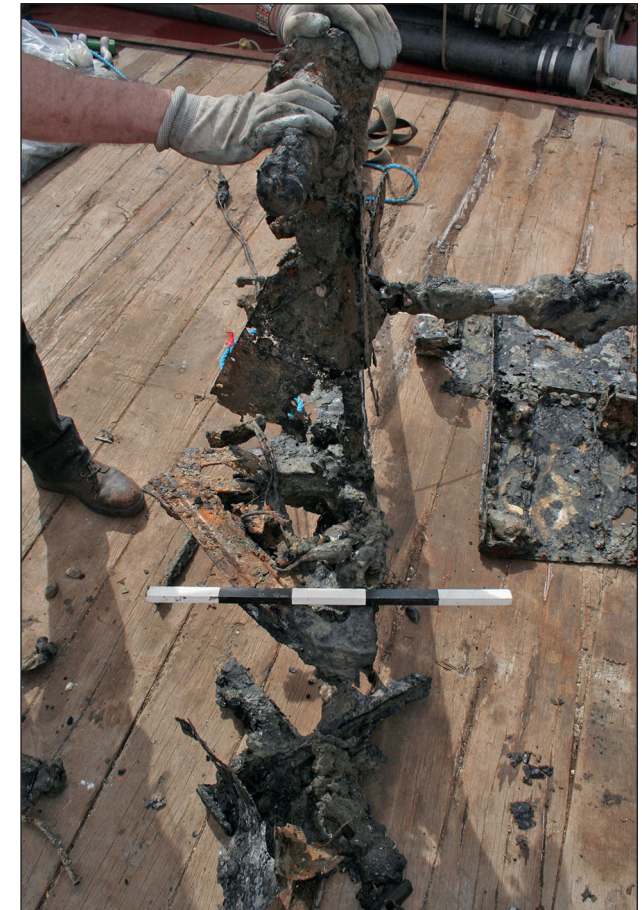
Plate 3: Starboard wing fragment- Rear spar fragment with piston for Youngman flap
