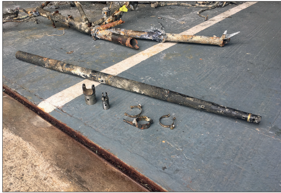
Plate 91: Cockpit tubes after disassembly © Tony Jupp
