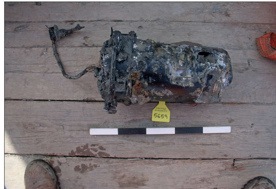
Plate 25: Distant Reading (D/R) Compass
