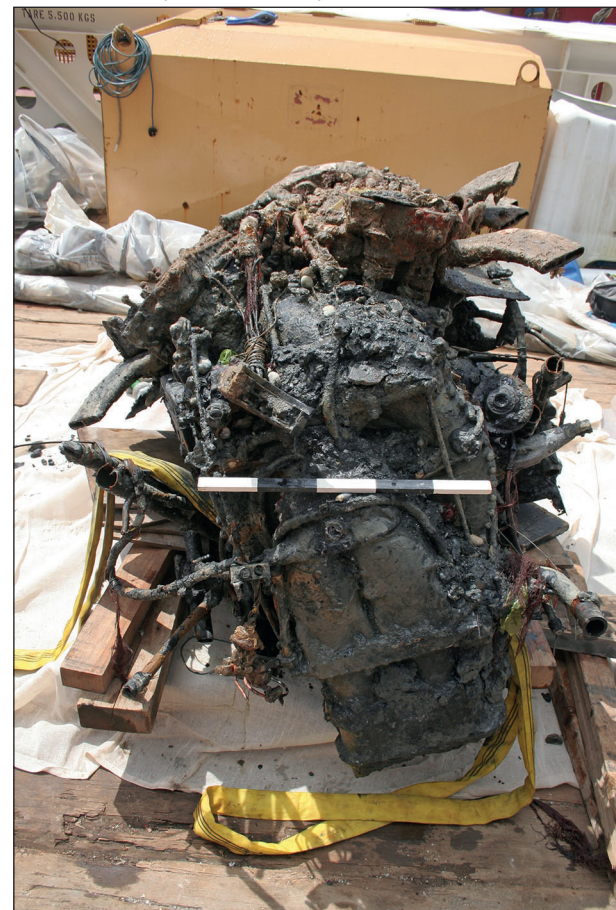
Plate 15: Rolls Royce Merlin 32 engine- rear of engine showing supercharger
