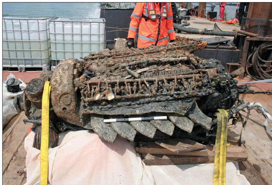
Plate 14: Rolls Royce Merlin 32 engine- port side showing rocker covers and 6 intact exhaust manifolds
