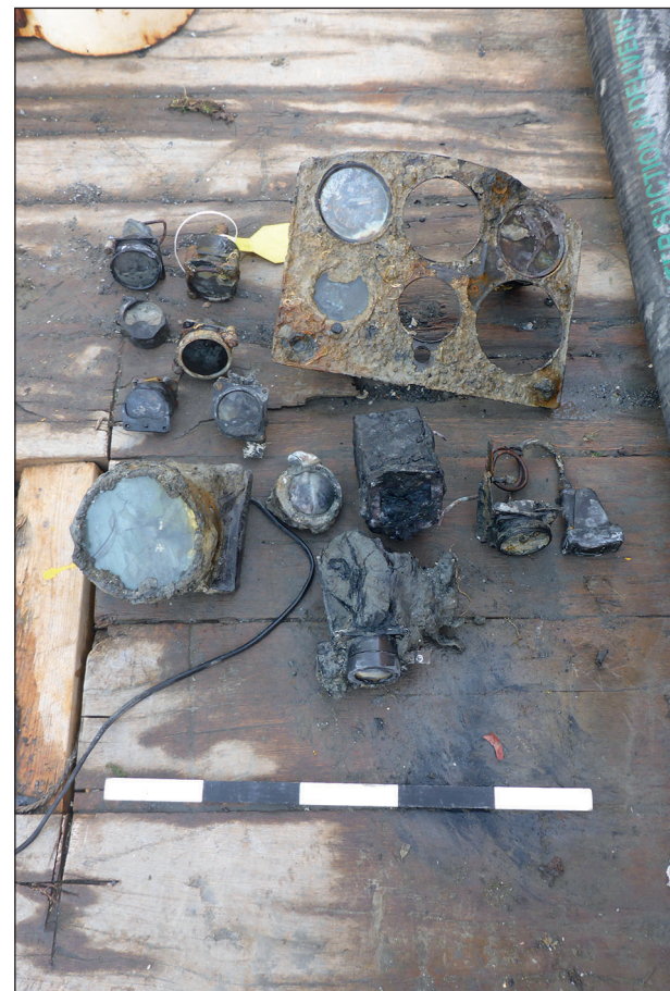
Plate 80: Radium painted dials in the Blind flying panel
