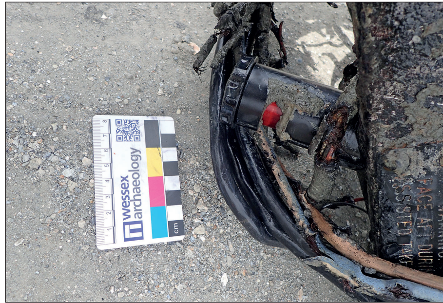
Plate 62: Cockpit light and warning label
