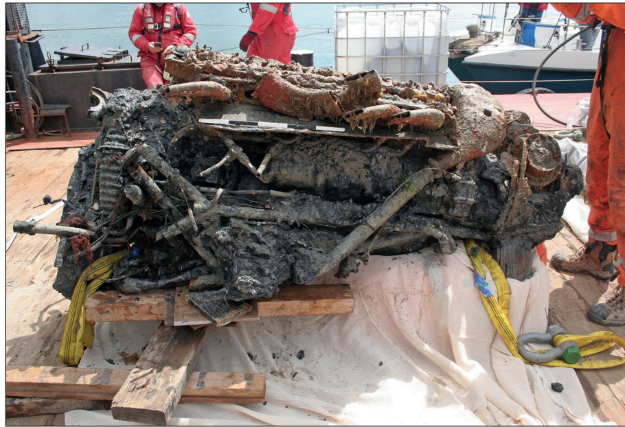
Plate 16: Rolls Royce Merlin 32 engine- starboard side showing damaged exhaust manifolds
