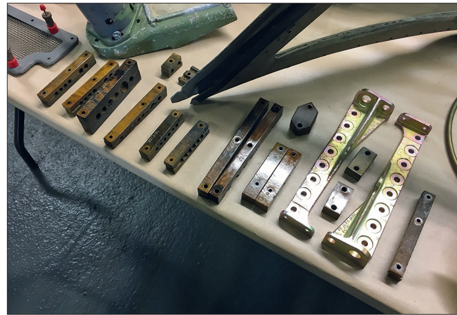
Plate 12: Tufnol and Bakelite blocks, pipe clamps and fittings recovered from the Barracuda and conserved by FAAM © Tony Jupp
