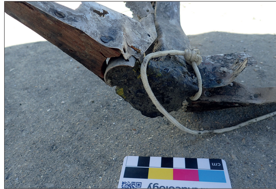
Plate 97: Rudder ribs with wooden spacers
