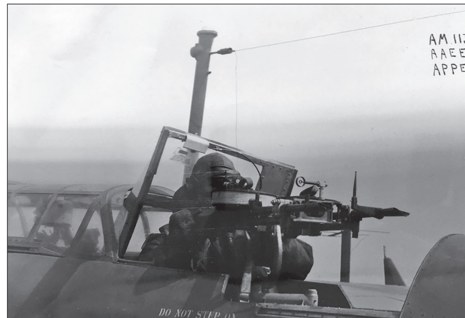
Plate 45: TAG with Vickers K Gun showing flat pan magazines on top (National Archives, AVIA18/784)
