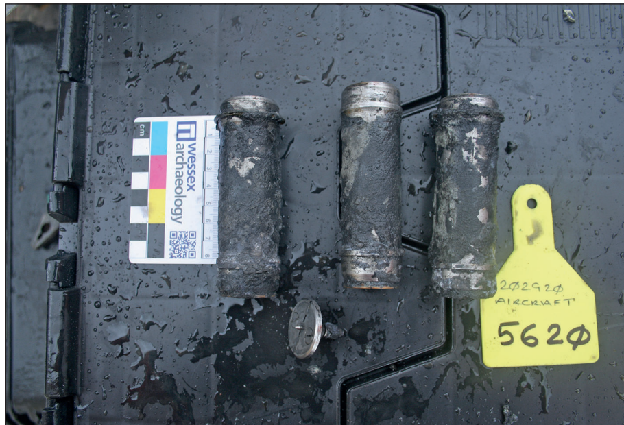
Plate 19: Coffman starter cartridges after EOD clearance
