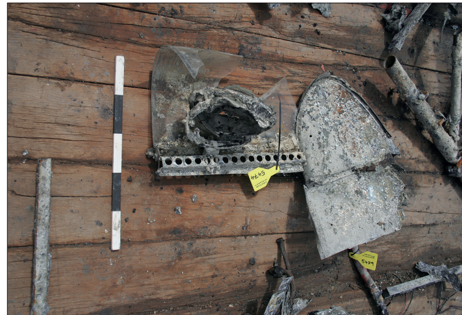
Plate 35: Landing light and Perspex cover
