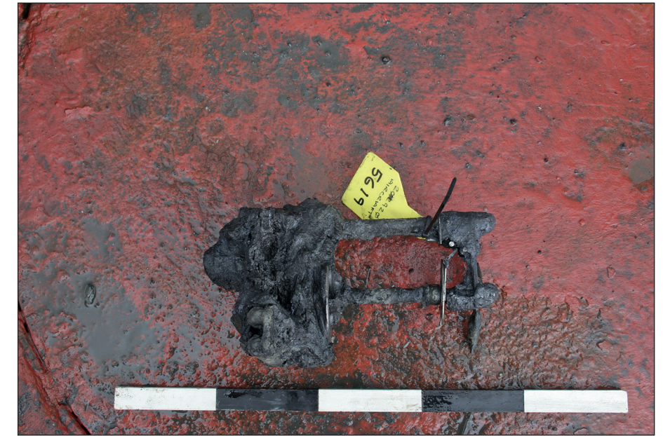
Plate 18: Coffman starter cartridge holder after cartridges removed for EOD clearance
