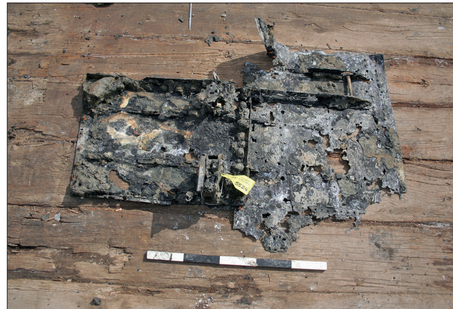
Plate 5: Starboard wing fragment- inner face of lower wing skin with stiffeners
