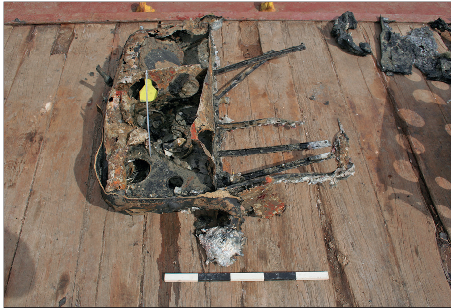
Plate 1: Starboard wing fragment- inboard fuel tank
