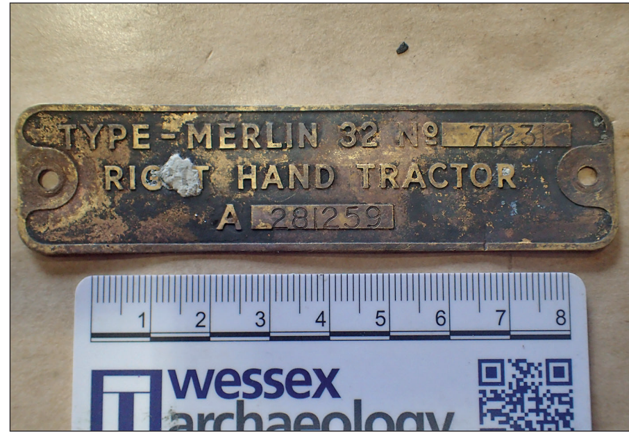
Plate 22: Identification plate for Merlin 32 engine
