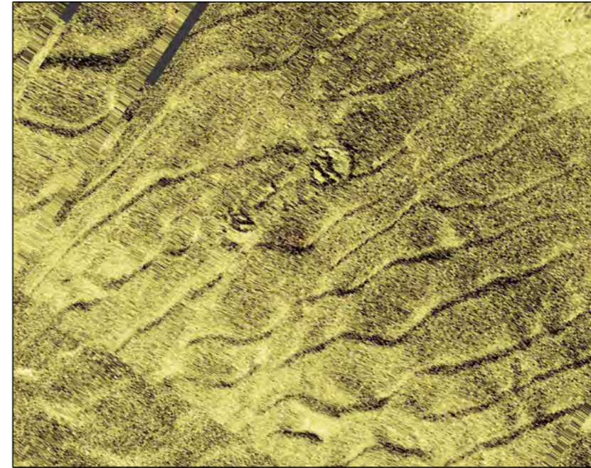
Plate 3. Site 7049: Site formed by angular dark reflectors, interpreted as a possible wreck measuring 21 x 7.5m
