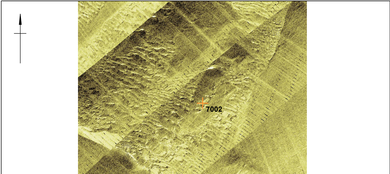
A: WA7002 : Probable wreck site measuring 31m x 7.2m x 0.3m. Structure found in an area where other objects have been identified in previous assessments (2007).
