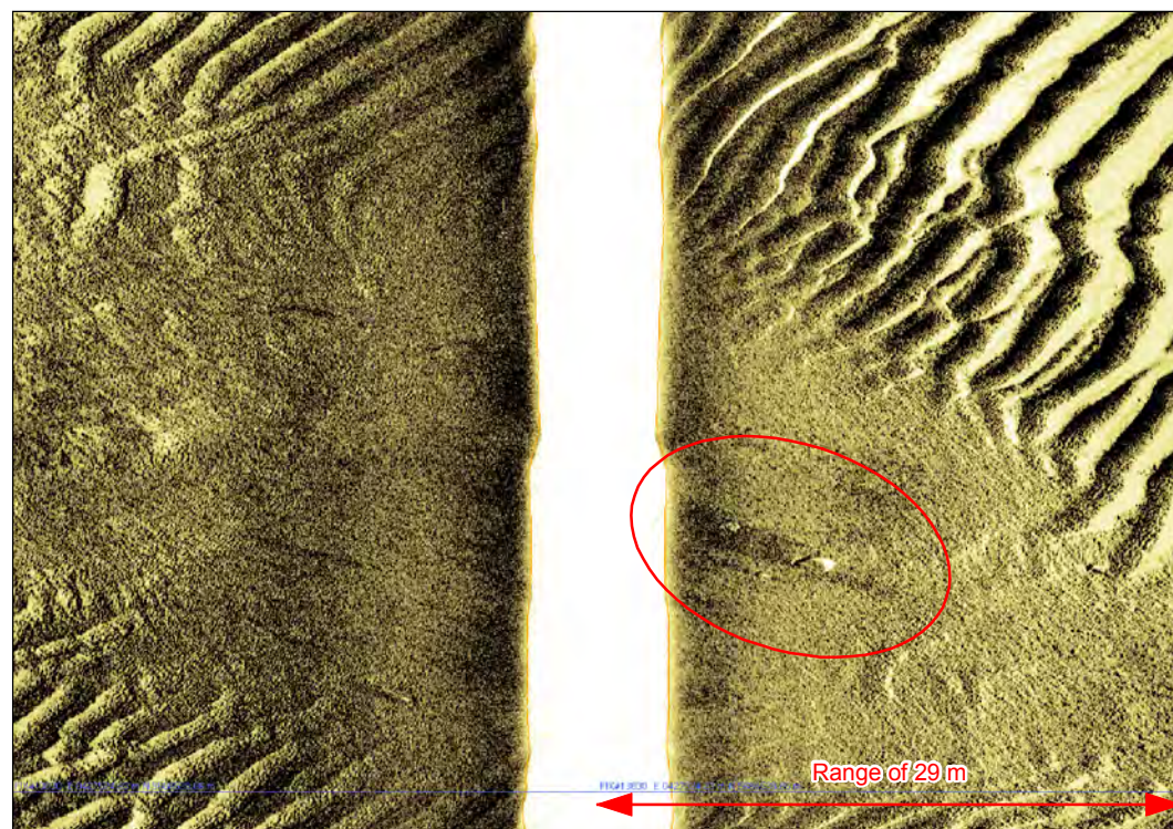
Sidescan sonar image of debris field 7426 (MAG_4979): 12.5 m x 4.6 m 2.3 m
