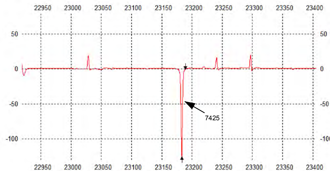
Magnetometer profile (negative peak) of 7425 measuring 134 nT in total
