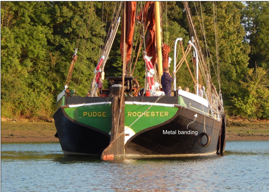
Plate 2: Metal banding on a restored Thames Sailing Barge, Pudge . Photo courtesy of the Thames Sailing Barge Trust.
