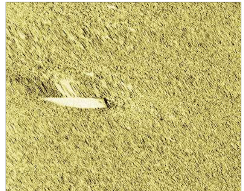
Sidescan sonar image of dark reflector 7582 , measuring 3.2 x 2.5 x 0.7 m
