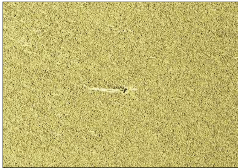
Sidescan sonar image of ferrous debris 7737 , measuring 1.5 x 1.0 x 0.5 m
