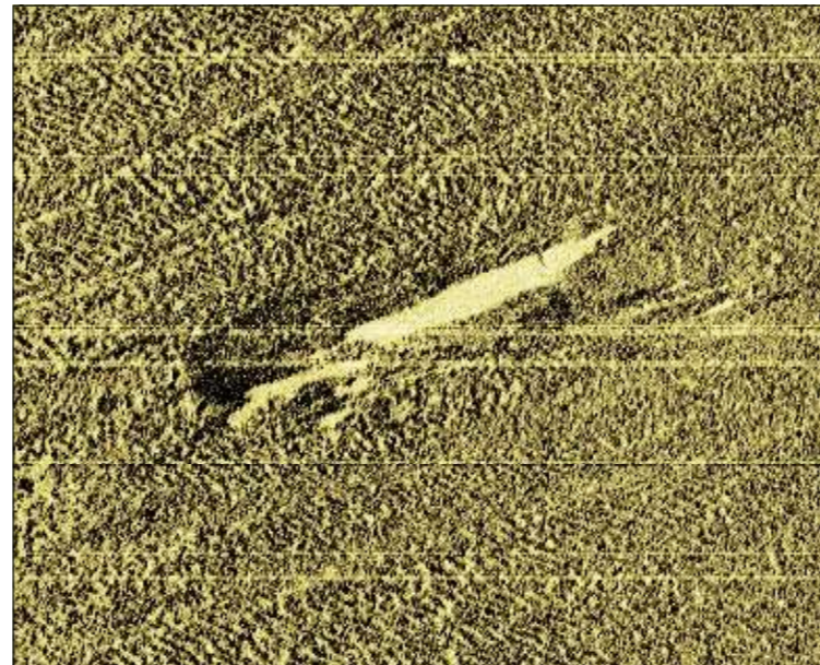
Sidescan sonar image of seabed disturbance 7142 , measuring 10.3 x 7.6 x 0.1 m
