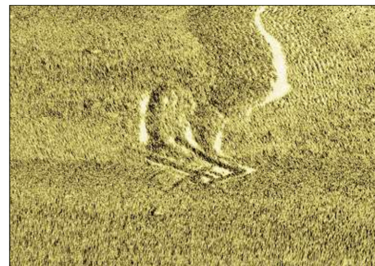
Sidescan sonar image of seabed disturbance 7705 , measuring 15.2 x 5.6 x 0.1 m
