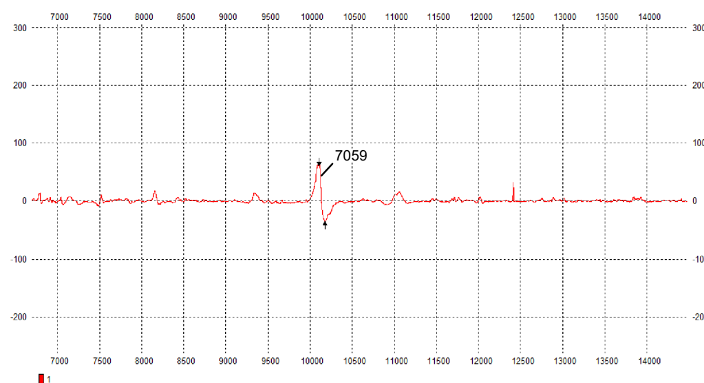
Magnetic profile of 7059 measuring 122 nT
