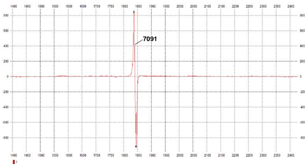
Magnetic profile of ferrous debris 7091 measuring 1782 nT
