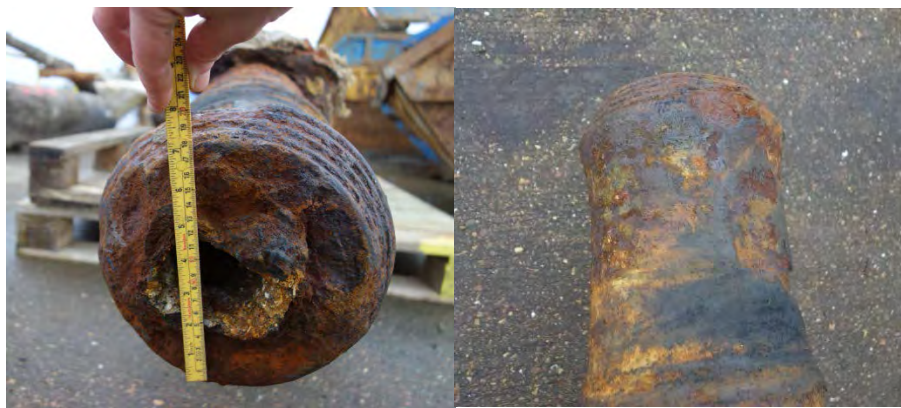
Figure 3 Bore and muzzle swell
