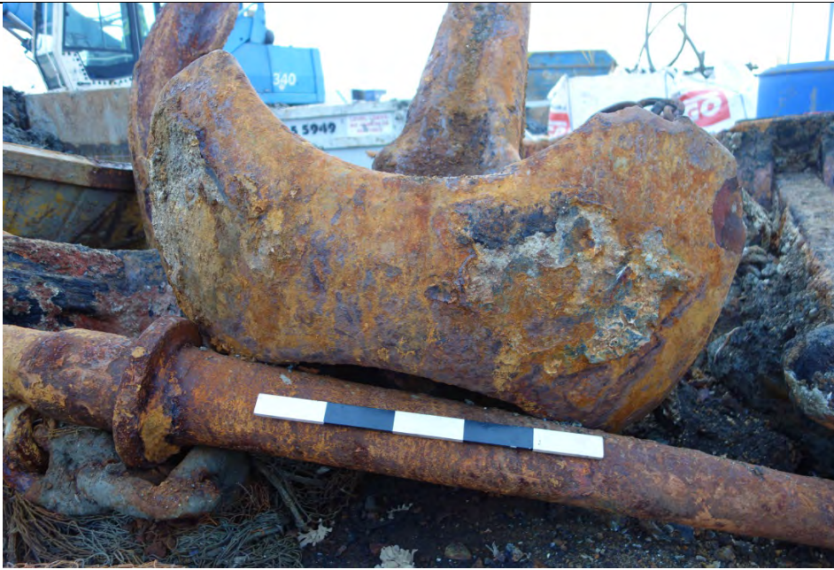
Detail of base/crown, showing concavity in the crown (stock is from another anchor)
