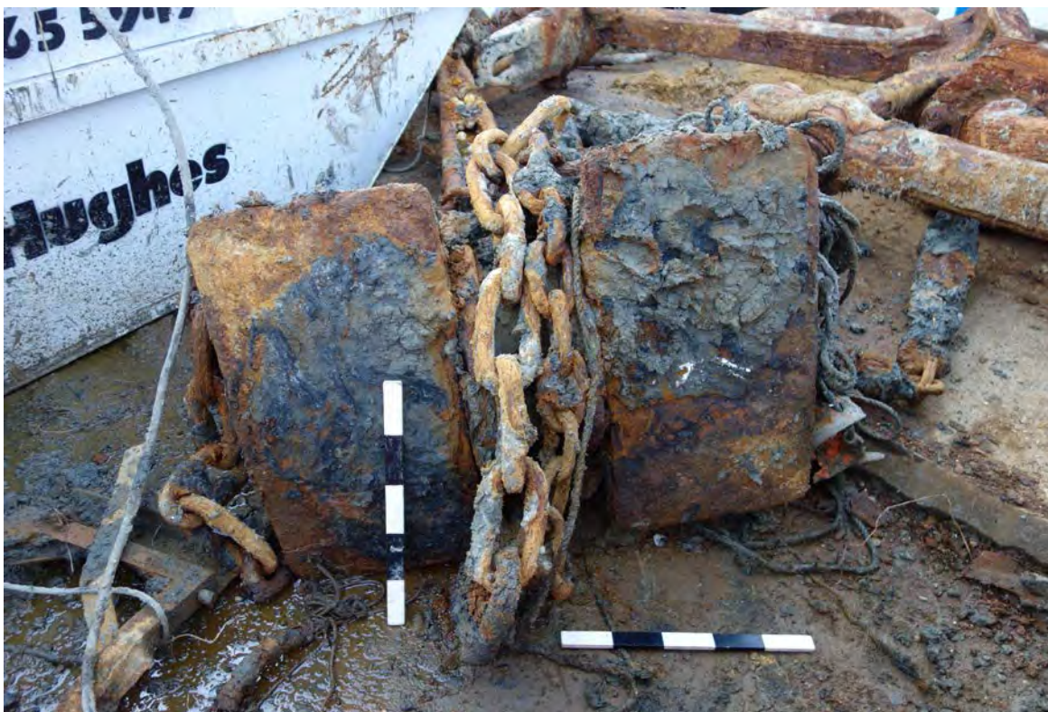
Tripping palms. The crown and head of the shank are obscured by the chain.
