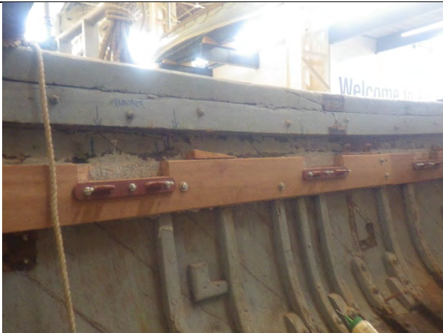
Rising timber. As seen (left) sits on top of the framing and is also the end of the internal frames.
