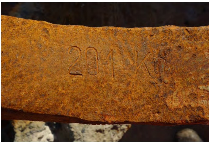
Anchor weight on the shank
