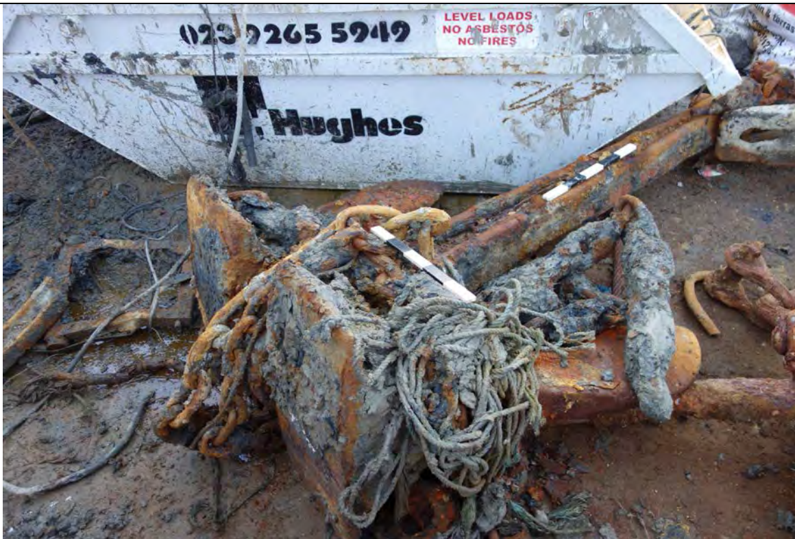
Side view showing the tripping palms and double plate girder shank
