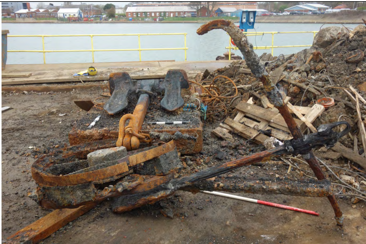
BWL9_0100 – The bent over arm can be seen facing the camera. An example of a stockless anchor can be seen in the background.
