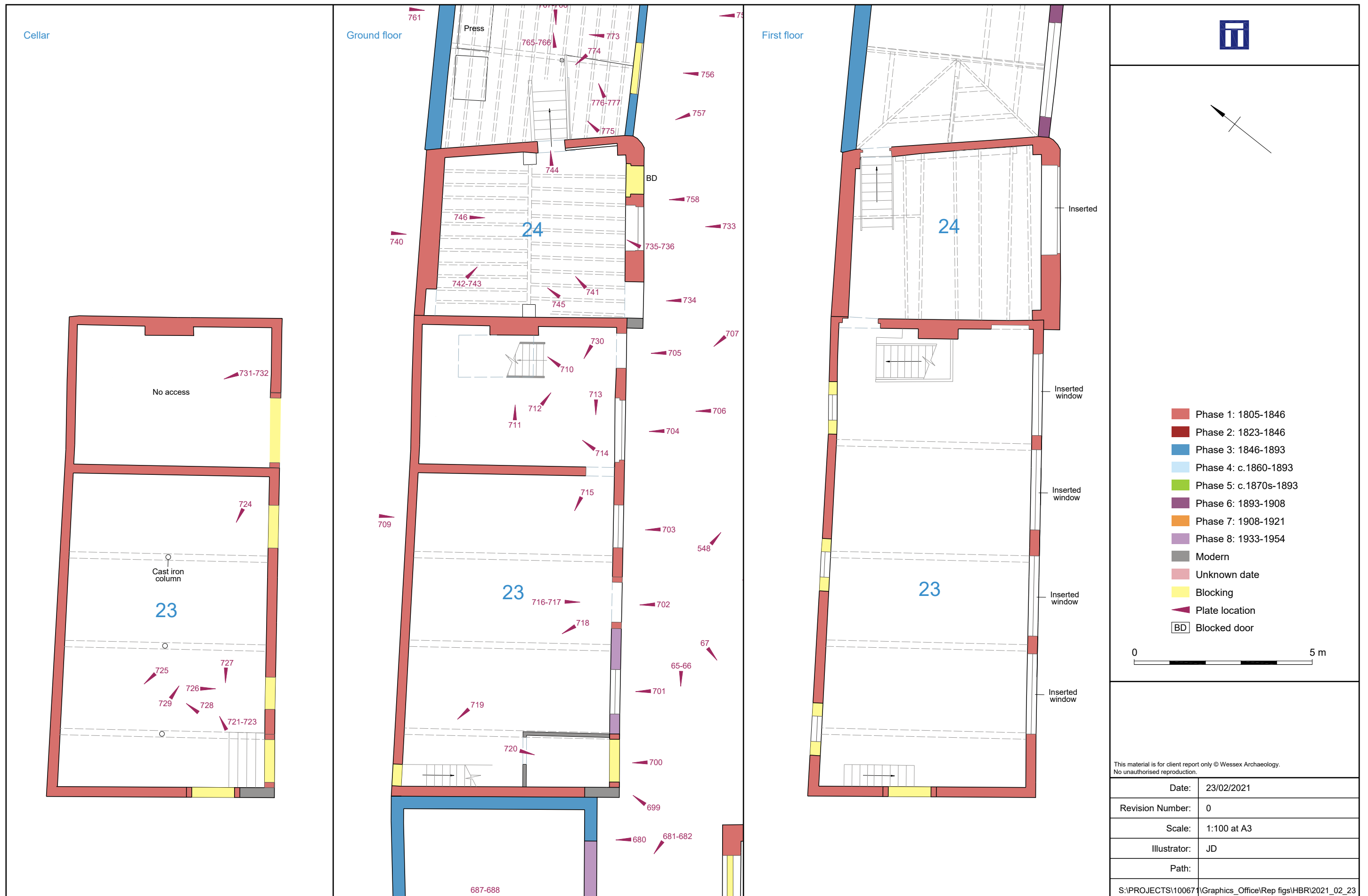
Phased plan and plate locations, buildings 23-24, cellar (building 23), ground floor and first floor (buildings 23-24)
