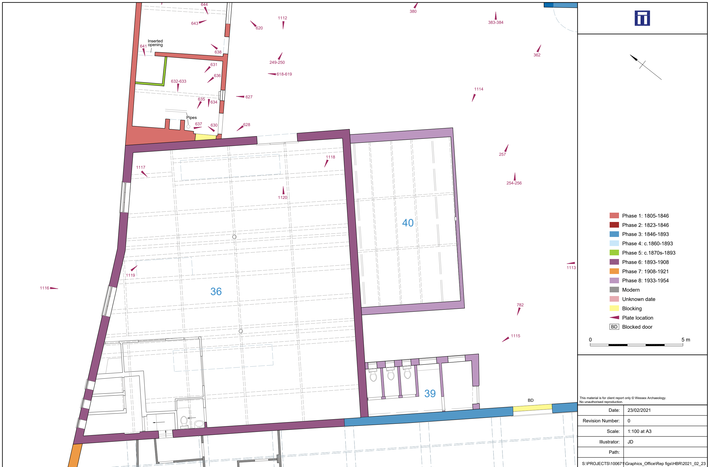
Phased plan and plate locations, buildings 19, 36, 39-40, ground floor
