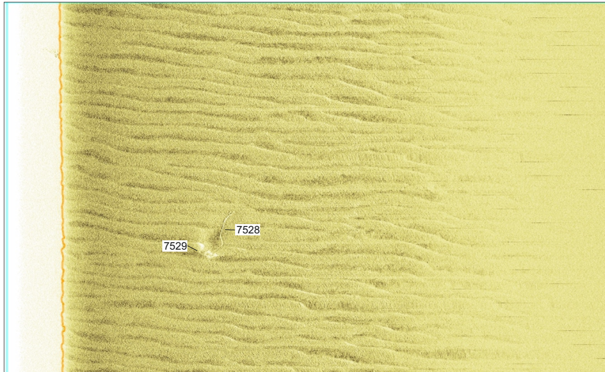
Sidescan waterfall image of rope/chain 7528, measuring 24.8 x 0.3 x 0.1 m
