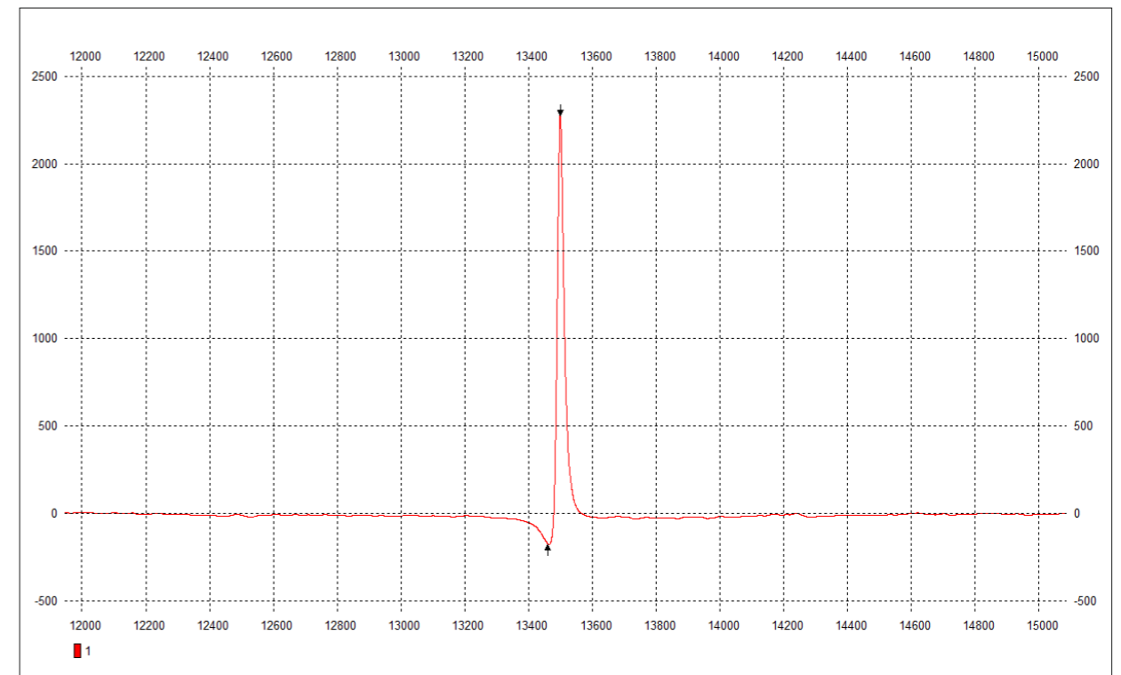
Marine magnetometer profile of anomaly 7486, 2474 nT
