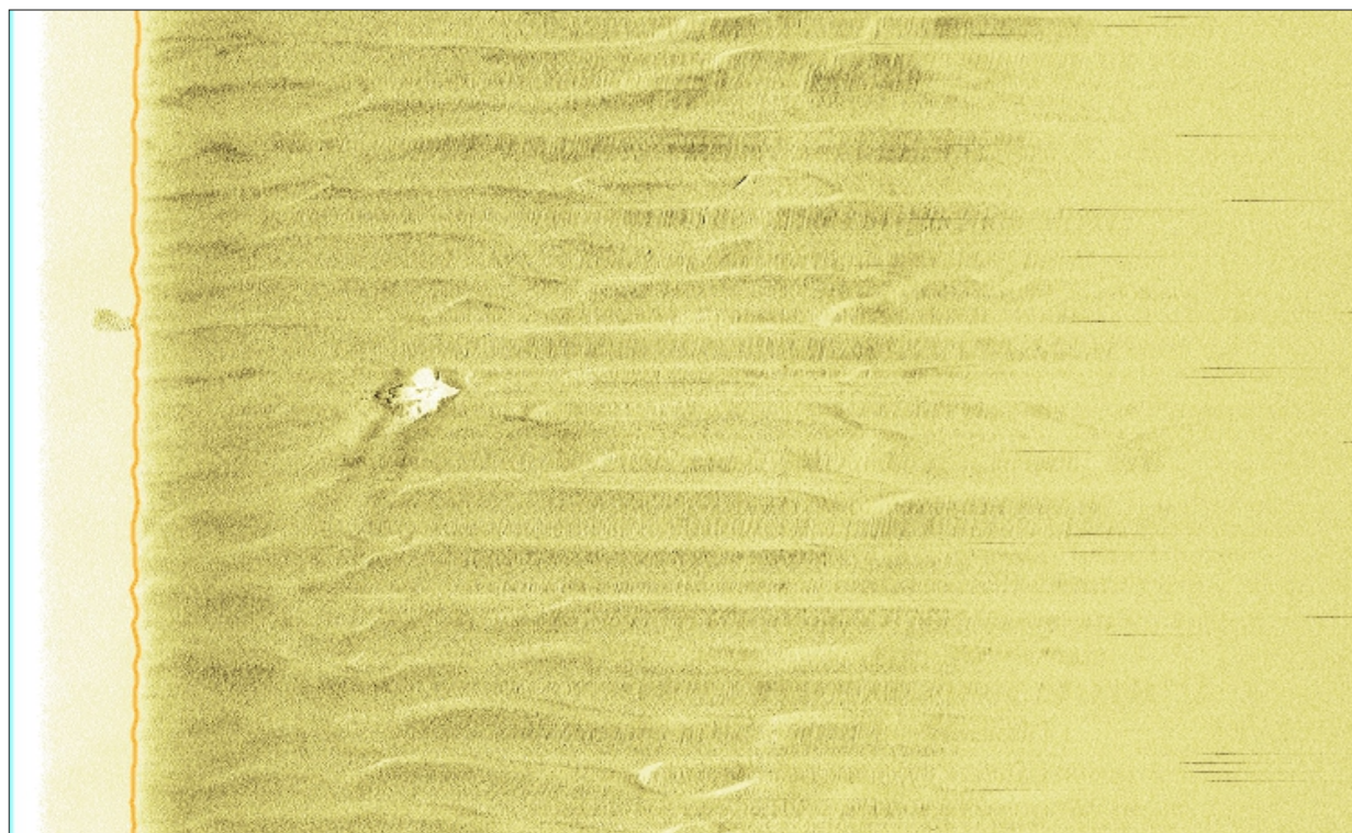
Sidescan waterfall image of debris 7182, measuring 9.5 x 2.7 x 1.6 m
