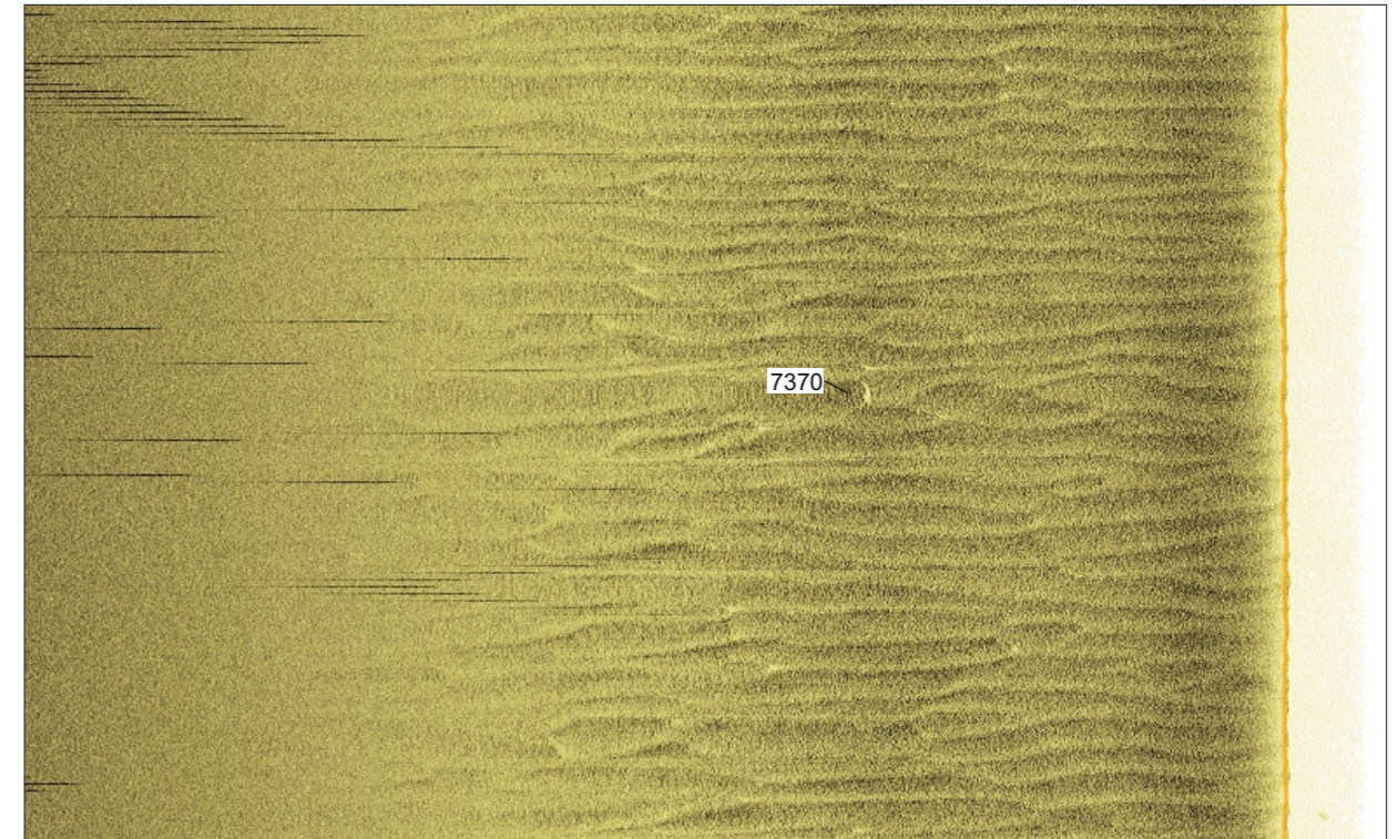
Sidescan sonar waterfall image of bright reflector 7370, measuring 4.1 x 1.0 m
