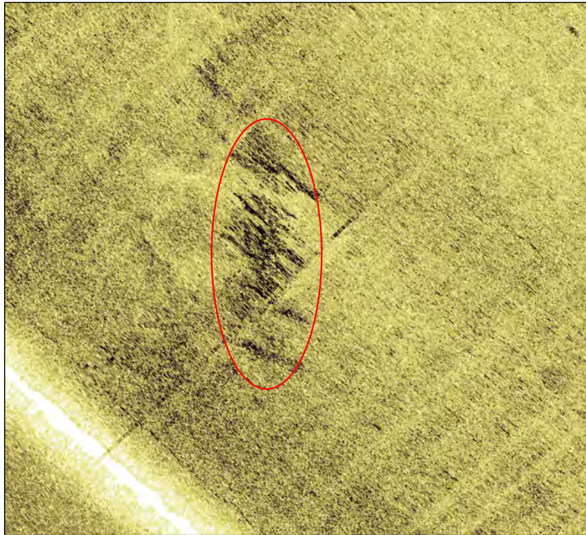
Sidescan sonar anomaly 3023: Wreck identified as an elongated patch of dark reflectors (21.5m x 12.1m)
