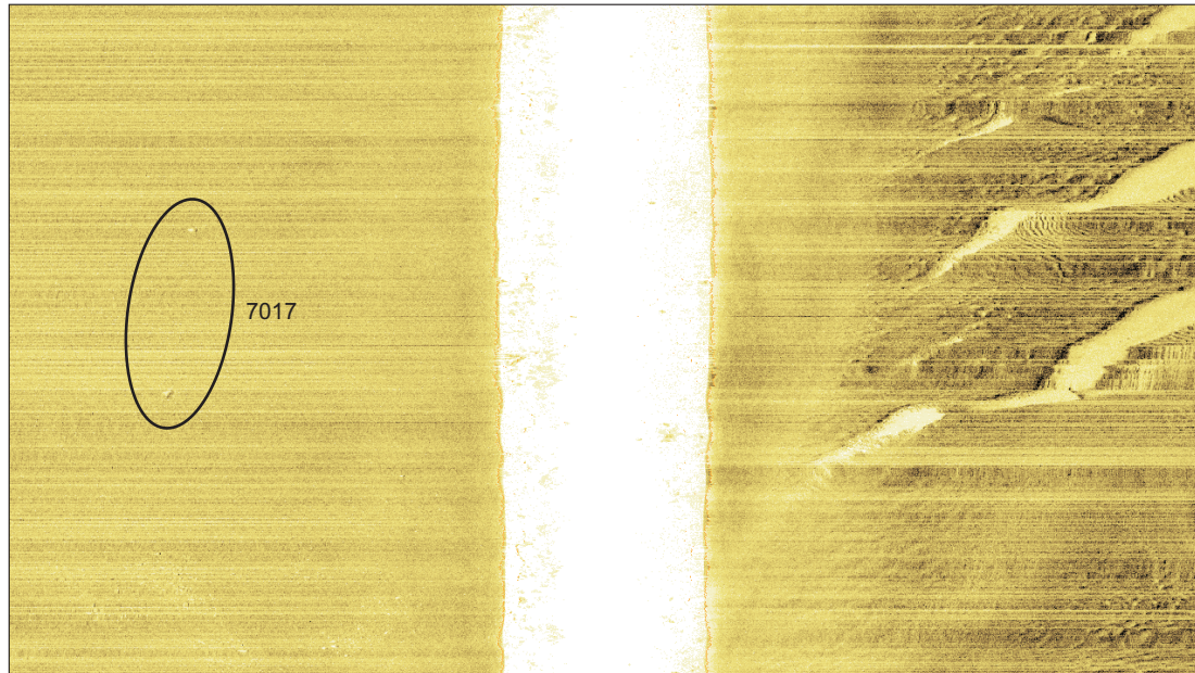
7017. Debris. Two objects 73m apart measuring 4.1m x 0.3m x 0.3m and 0.9m x 0.3m x 0.4m
