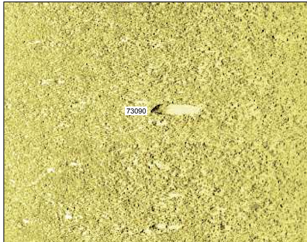
73090 - Small angled object with shadow, 1.3m x 0.4m x 0.3m, possible debris. No associated magnetic anomaly suggests non-ferrous material
