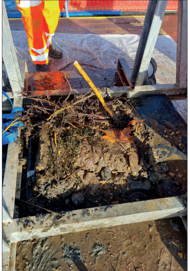
Figure 6: Example of organic debris recovered at 7030 (GS09)
