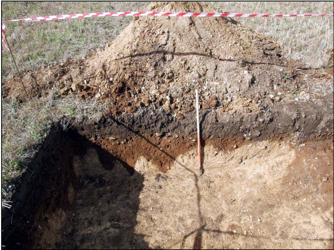
FIGURE 5a: MACHINE CUT GEO-TECH PIT AT SOUTHERN END OF TRENCH 7 SHOWING NATURAL GEOLOGY OVERLAID BY PLOUGHSOIL (701)
