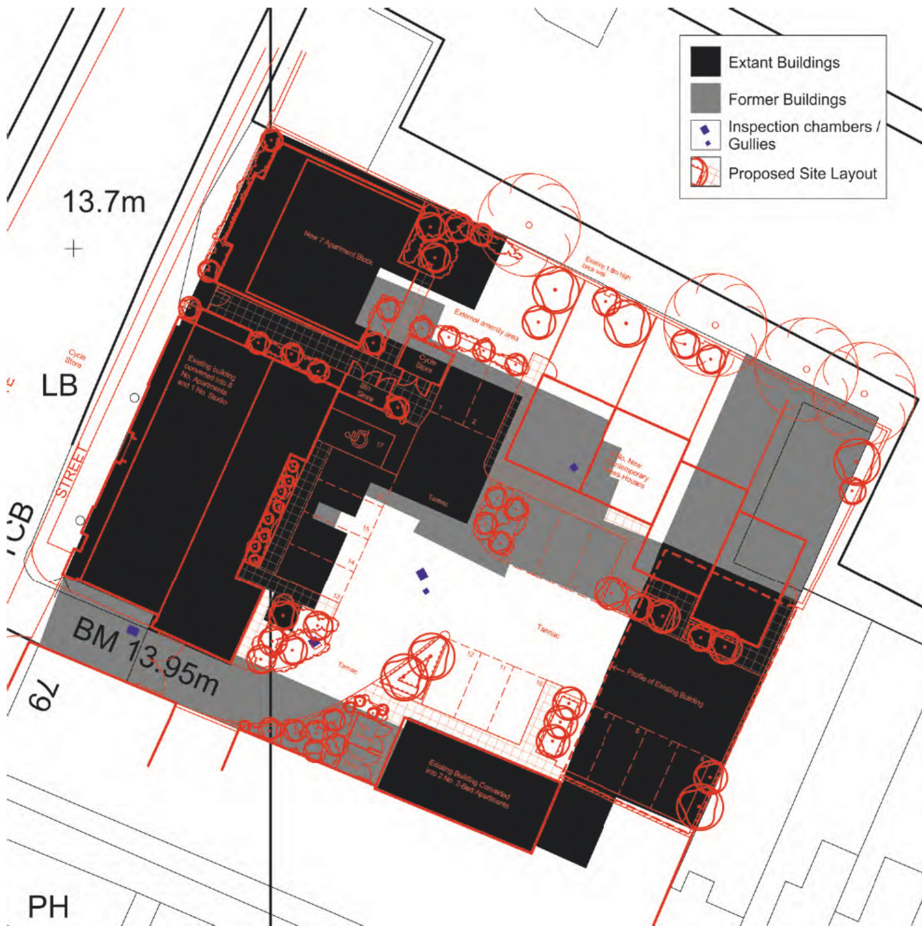
Figure 9: Disturbance plan overlain with proposed site layout, 1:250 @ A3
