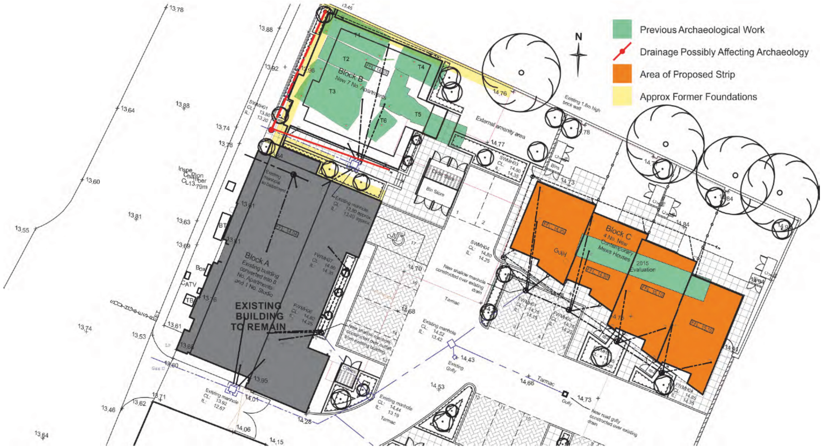
Figure 10: Proposed ground disturbance and proposed drainage routes, 1:200 @ A3
