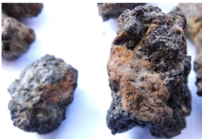
Figure 5 Close up of a fragment of vitrified material showing inclusions of oxidised ceramic.
