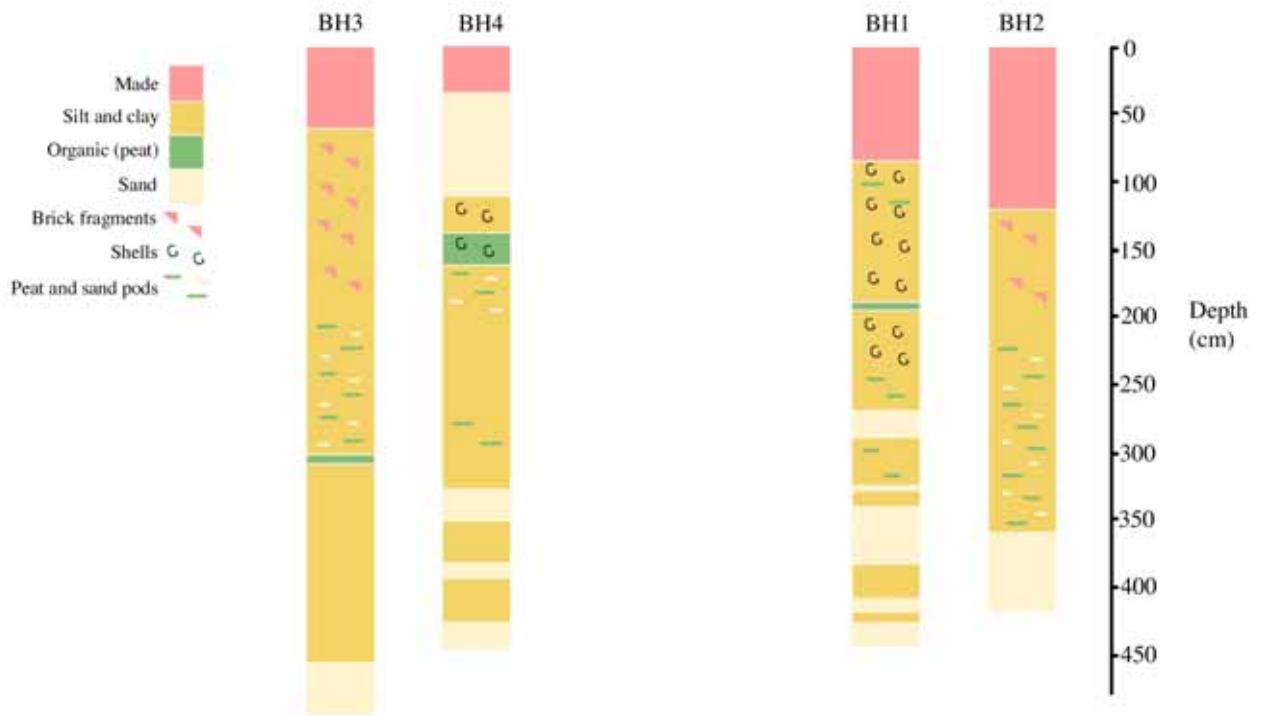
Simplified geology from BH1-4 SW-NE across the Cromwell Road Site
