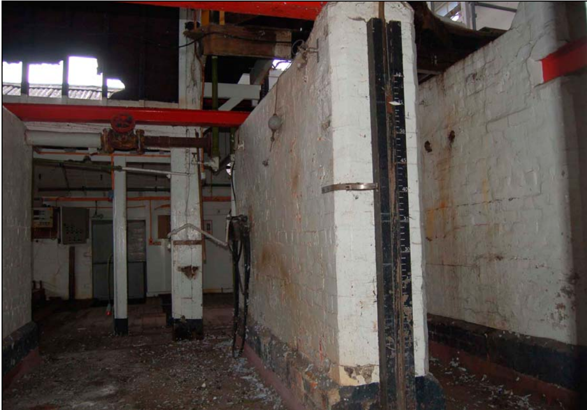
Plate 46 Level gauge for copper
