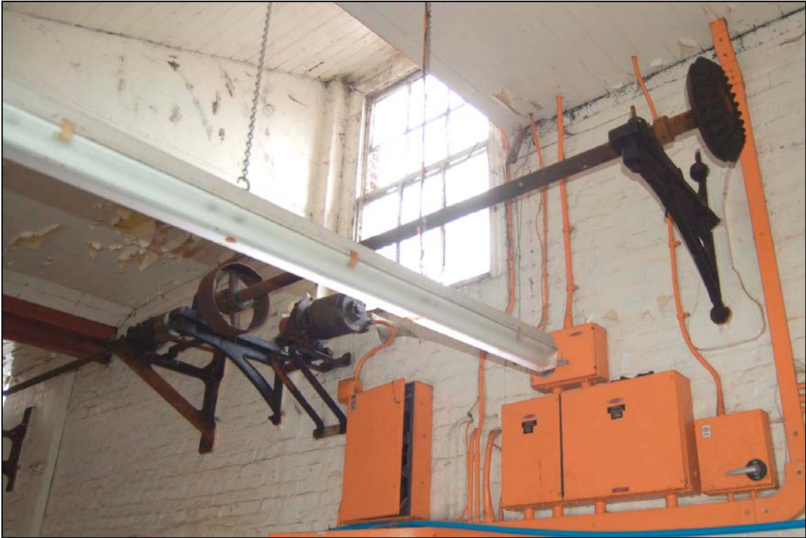
Plate 38 Moss Gear motor and gearing for vertical shaft
