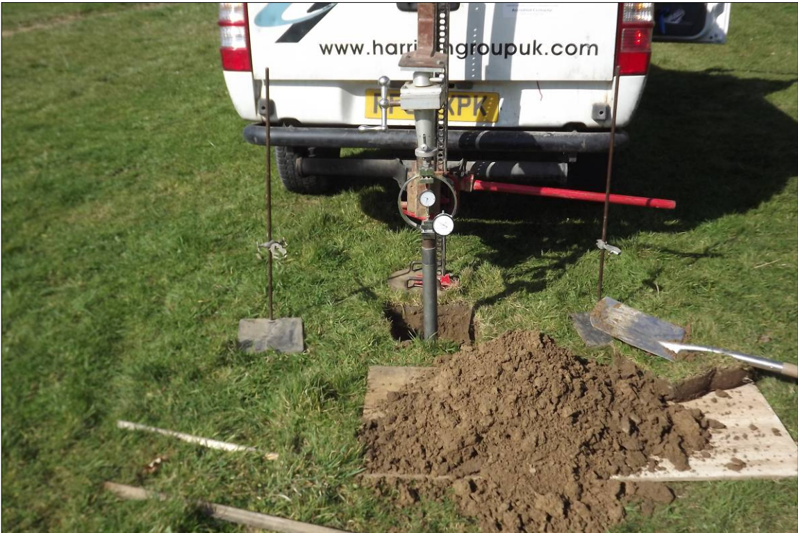
Plate 4. California Bearing Ratio test
