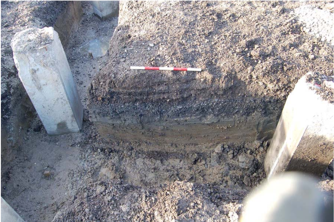
Plate 2 Typical section showing the varying layers of modern made ground and the underlying clay (0.5m scale bar)
