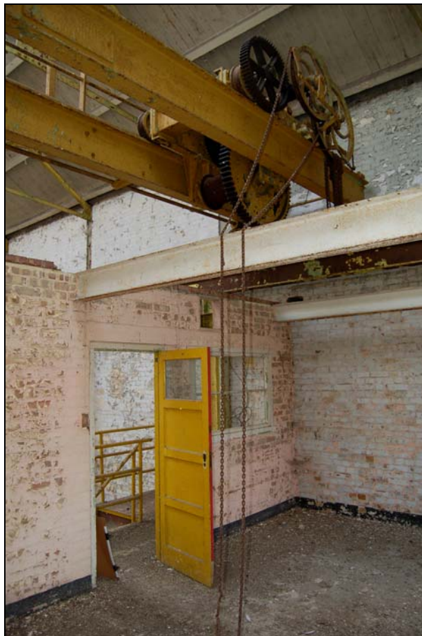
Plate 14 Detail of travelling crane manufactured by John Smith of Keighley
