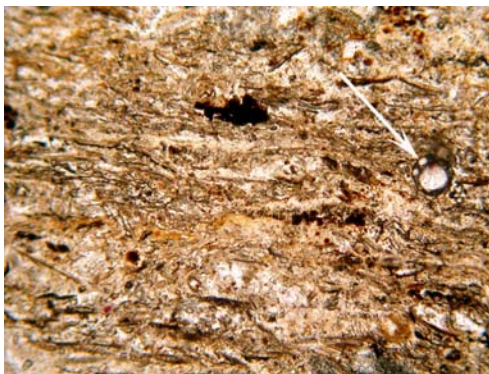
Figure 223: The Soil Micromorphology: as Figure 221; compact phytoliths-rich layer; note cross-section through silica-replaced 'straw' stem (arrow). PPL, frame width is ~1.00mm.
