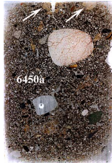
Figure 128: Soil micromorphology: scan of M11A (Context 6450; sub-unit 6450a), immediately below collapsed Roman wall 6449; note coarse mortar (arrows) at the top of the thin section (from 6449); mortar is present throughout – presumably weathered from nearby wall 6449 (see Figure 135 -Figure 140). Width is ~50mm.
