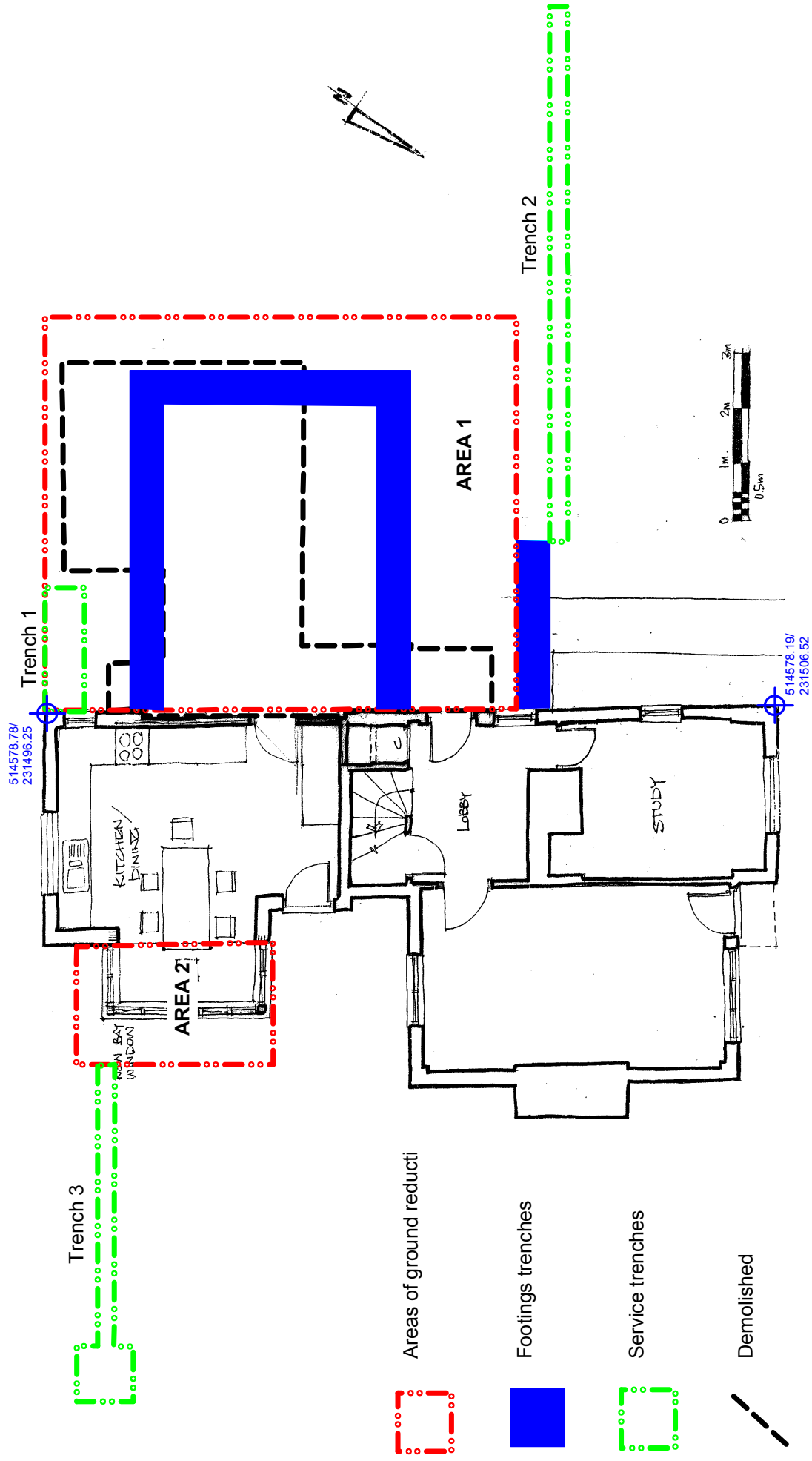
Plan showing location of development groundworks Base plan courtesy of Pentangle Design
