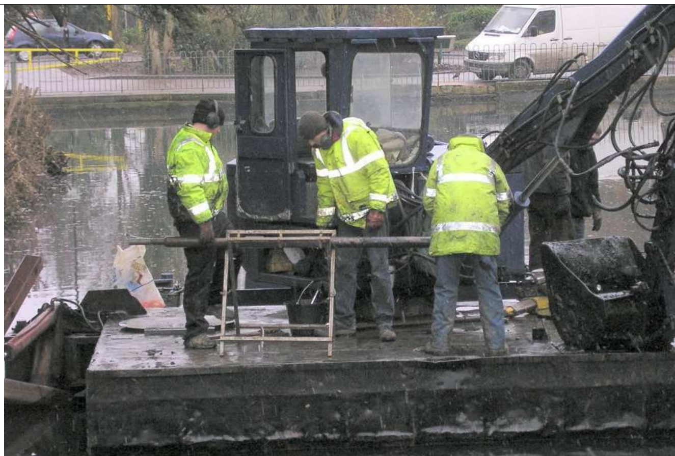
Plate 4: Extracting the core from the sampler in the SW arm of the moat
