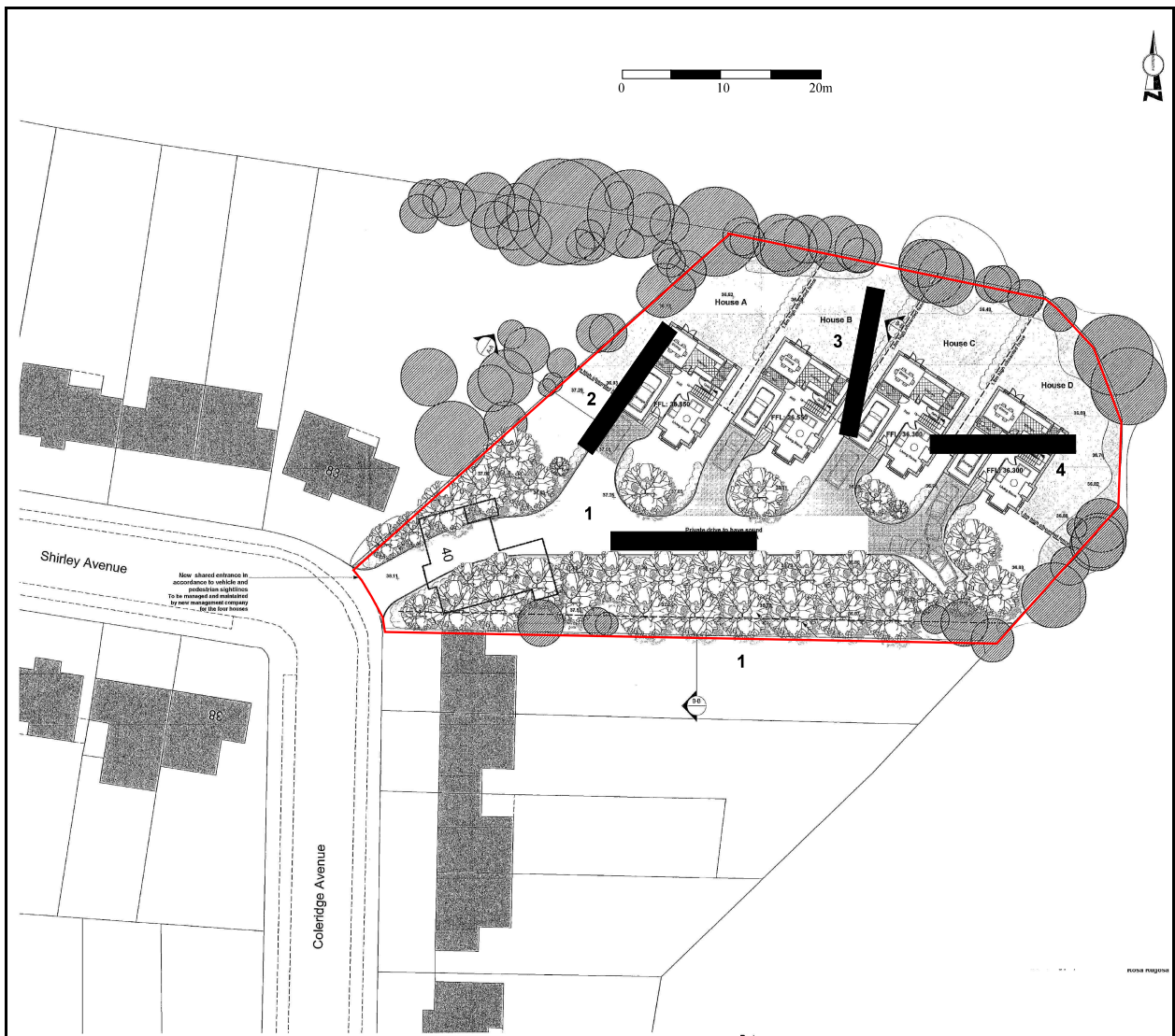
Fig. 4 Development and trench location Plan
