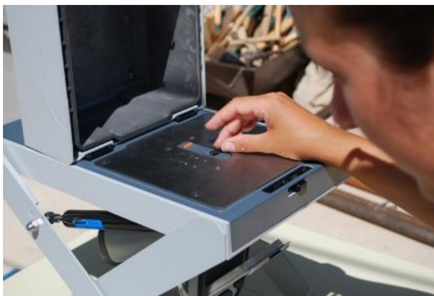
Figure 9.14. Placement of artefact over analyser window in tungsten-lined portable stand (pXRF below).
