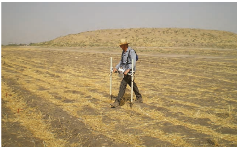
Figure 5.1. Fluxgate gradiometry survey over the area southeast of the mound.
