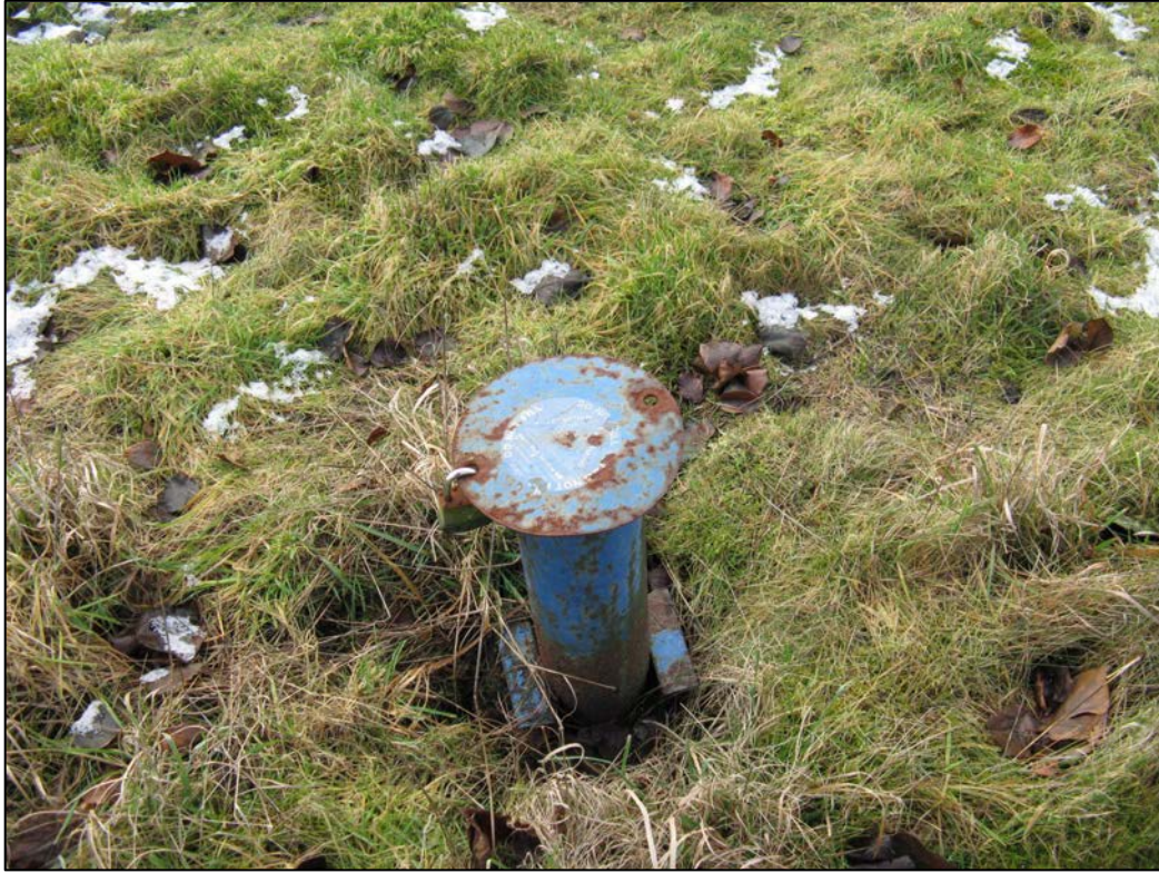
Figure 17: Groundwater monitoring point in Area A
