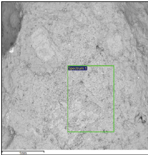
Back-Scattered SEM image of Sample 3 (AAL15 (304) <3> XRF), probably a weathered granite (rhyolite?). Area of EDS analysis is shown in Green
