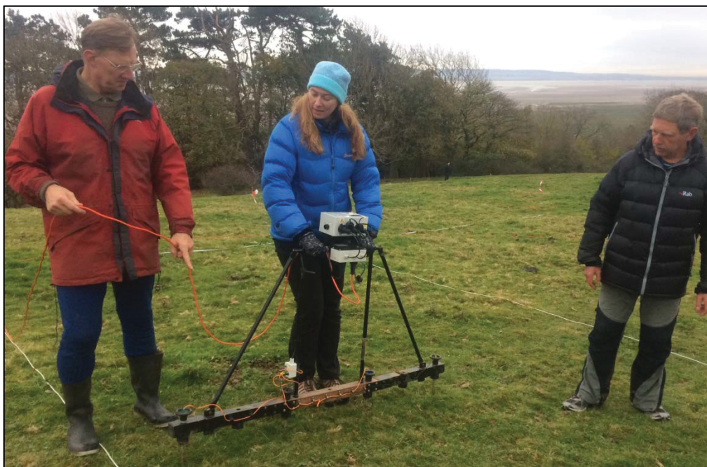
Earth electric resistance survey using a Geoscan RM15D and MPX15
