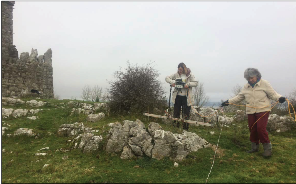
Earth electric resistance survey around the outcropping bedrock near the Summer House
