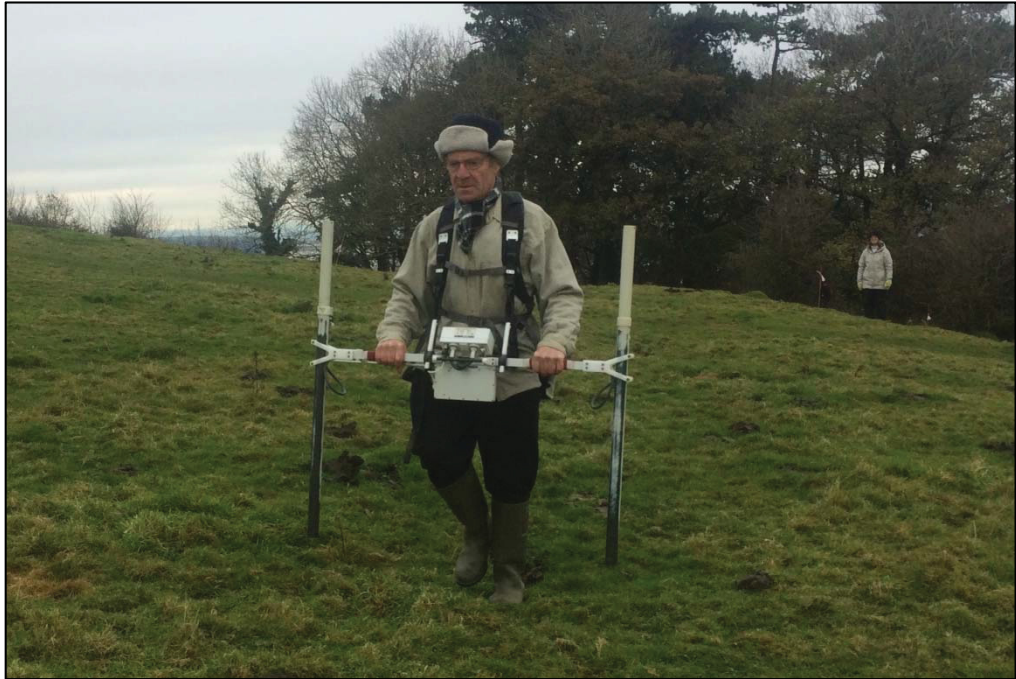
Geomagnetic survey using a Bartington Grad601-2
